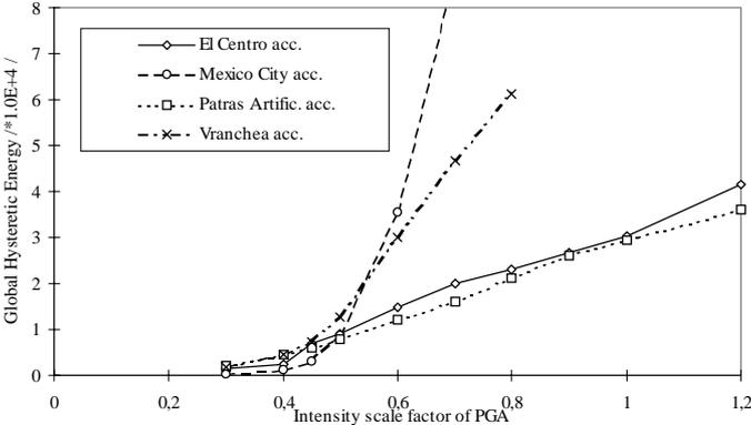
**Fig.3 Vulnerability Functions for Global Hysteretic Energy - R/C Frame -BGSC**
