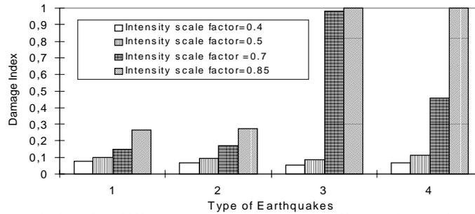
**Fig.2 Damage index for different earthquakes and different intensity scale factor - R/C Frame -EC8**
