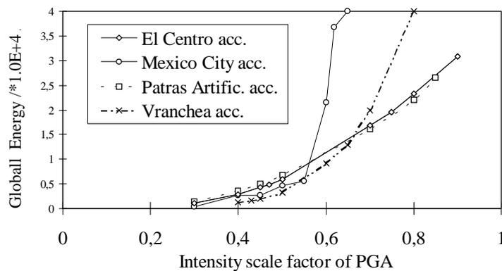
**Fig.1 Vulnerability Functions for Global Hysteretic Energy - R/C Frame - EC8**
