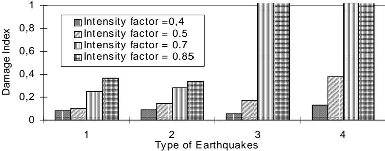
**Fig.4 Damage index for different earthquakes and different intensity scale factor for BG R/C Frame 1- art. acc.Patras; 2- acc. El Centro; 3-acc. Mexico City; 4-acc. Vrancea**
