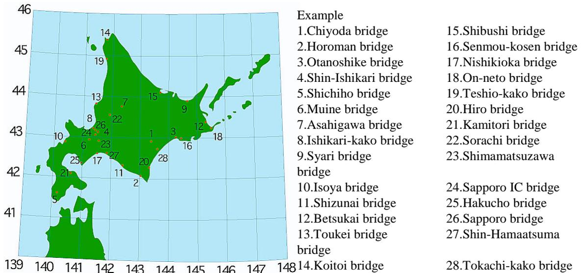
**Figure 3-1-1 Arrangement of strong-motion seismographs installed by 1993**
