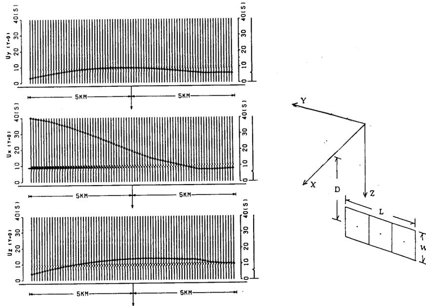
Figure 5: Time-domain responses for surface velocities  $u_z$ ,  $u_x$ , and  $u_y$  at 79 sites equally spaced along the x axis of the Half-Space due to a moving fault ( i.e., dip angle  $\delta = 90^\circ$ , rake angle  $\lambda = 180^\circ$ , strike angle  $\phi = 90^\circ$ ) at  $(x = 6\text{km}, -13.5\text{km} \leq y \leq -7.5\text{km}, 9\text{km} \leq z \leq 11 \text{ km})$ . Rise time is 2.0sec and rupture velocity is 2.8km/sec.
