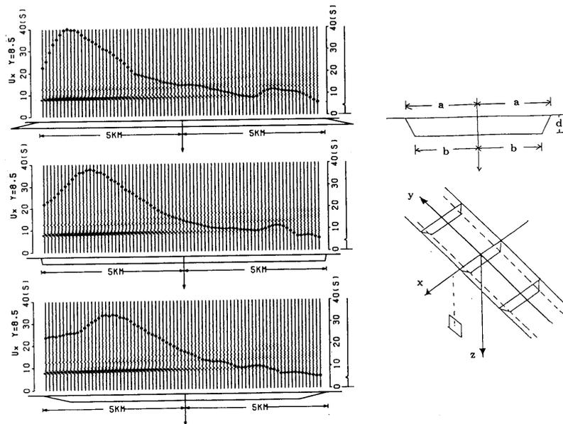
Figure 8: Effect of shape of 2-D basin edge on time-domain responses for fault-normal component surface velocity  $u_x$  along the  $y=8.5\text{km}$  due to a double couple force( i.e., dip angle  $\delta = 90^\circ$ , rake angle  $\lambda = 180^\circ$ , strike angle  $\phi = 90^\circ$ ) at  $(x=6\text{km}, y=0\text{km}, z=10\text{km})$ . Rise time is 1.0sec.
