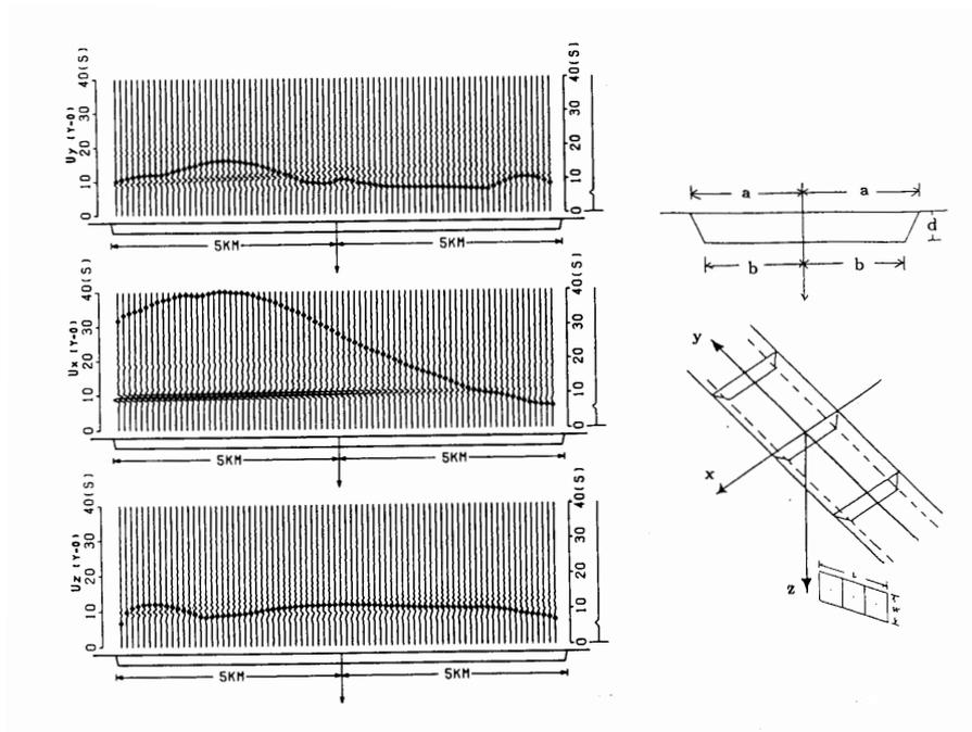
Figure 7: Time-domain responses for surface velocities  $u_z$ ,  $u_x$ , and  $u_y$  at 79 sites equally spaced along the x axis of Model B basin due to a moving fault ( i.e., dip angle  $\delta = 90^\circ$ , rake angle  $\lambda = 180^\circ$ , strike angle  $\phi = 90^\circ$ ) at  $(x = 6\text{km}, -13.5\text{km} \leq y \leq -7.5\text{km}, 9\text{km} \leq z \leq 11 \text{ km})$ . Rise time is 2.0sec and rupture velocity is 2.8km/sec.
