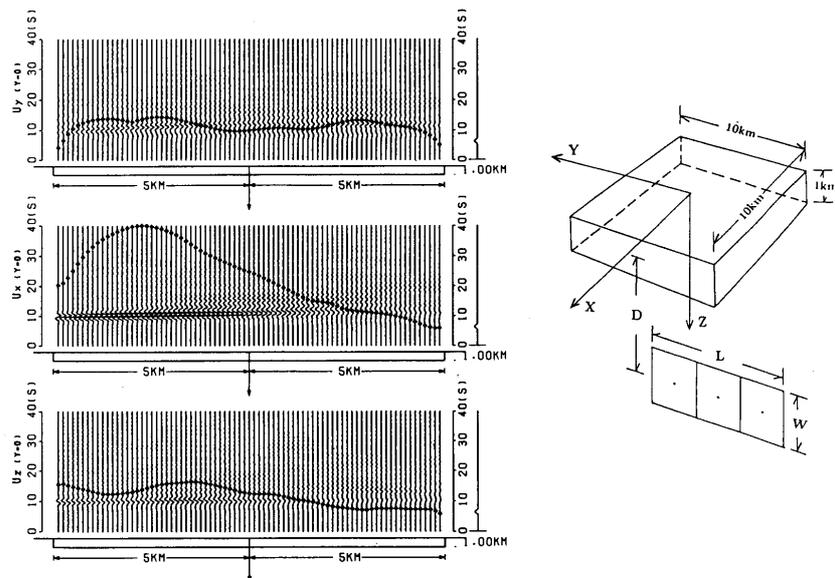
Figure 6: Time-domain responses for surface velocities  $u_z$ ,  $u_x$ , and  $u_y$  at 79 sites equally spaced along the x axis of the 3-D sedimentary basin due to a moving fault ( i.e., dip angle  $\delta = 90^\circ$ , rake angle  $\lambda = 180^\circ$ , strike angle  $\phi = 90^\circ$ ) at  $(x = 6\text{km}, -13.5\text{km} \leq y \leq -7.5\text{km}, 9\text{km} \leq z \leq 11 \text{ km})$ . Rise time is 2.0sec and rupture velocity is 2.8km/sec.
