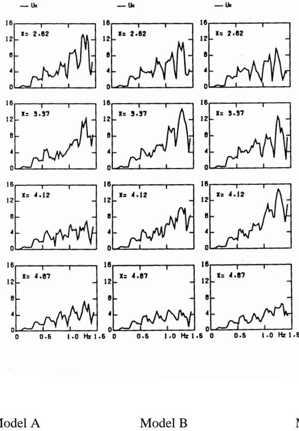
Figure 9: Amplitude characteristics of transfer functions for fault-normal component surface velocity  $u_x$  along the  $y=8.5\text{km}$  of 2-D basin model due to a double couple force. The fault parameters are the same as shown in Figure 8.
