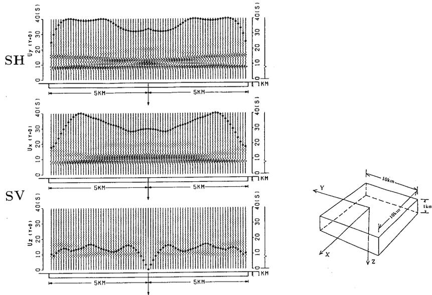
Figure 3: Time-domain responses for surface displacements at 79 sites equally spaced along the  $x$  axis of the 3-D sedimentary basin due to vertically propagating plane SH or SV waves. Source time function is a Ricker wavelet with a characteristic period of 2.0 sec.
