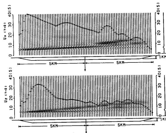
Figure 4: Time-domain responses for surface displacements  $u_z$  and  $u_x$  at 79 sites equally spaced along the  $x$  axis of the 3-D sedimentary basin due to a single point source excited in the  $x$  direction located at  $(x=6\text{km}, y=0, z=5\text{km})$ . Source time function is a Ricker wavelet with a characteristic period of 2.0 sec.
