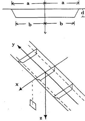
Figure 2: 2.5-D sedimentary basin model.
