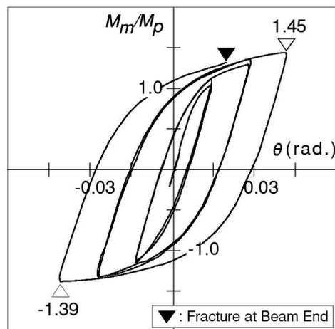
Figure A1.3: Beam end moment vs. relative rotation of beam end connection relationship
