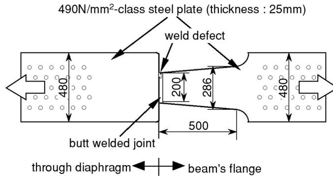
**Figure A3.1: Specimen configuration of tension test**
