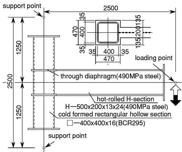
**Figure A1.1: Specimen configuration and loading condition**
