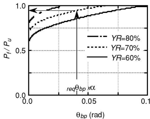
Figure 3: Flange force vs. plastic end rotation angle of beam relationships
