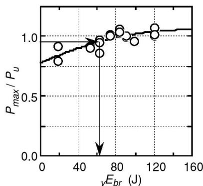
**Figure 4: Relationships between joint strength and fracture toughness**
