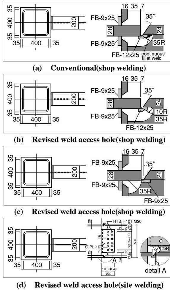
Figure A1.2: Detail of joint
