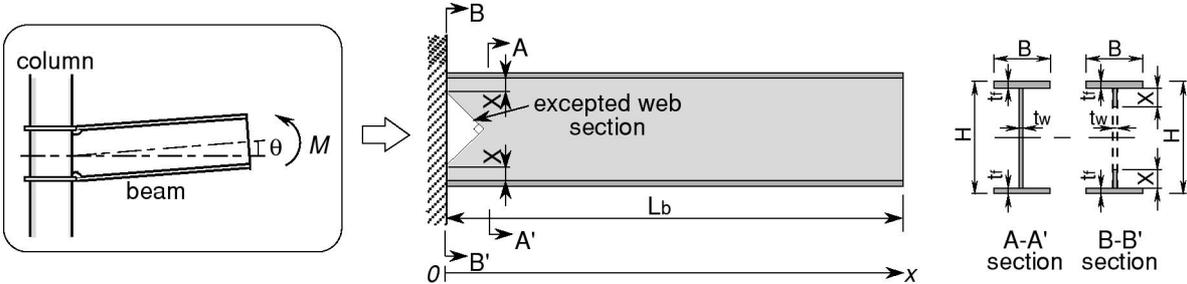
Figure A2.1: Configuration of CDC method model
