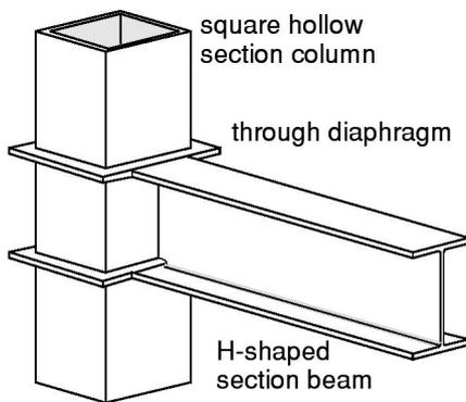
Figure 2: Typical type of beam-to-column connections
