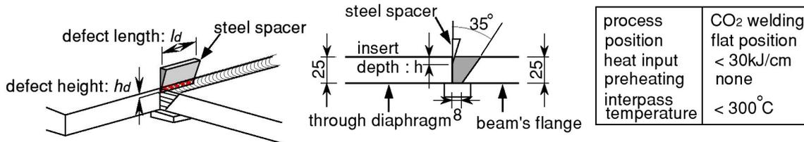
**Figure A3.2: Location of defect**
