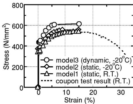
**Figure A3.4: Stress-strain models**
