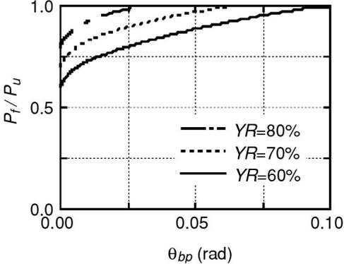
Figure A2.2: Flange force vs. plastic end rotation angle relationships
