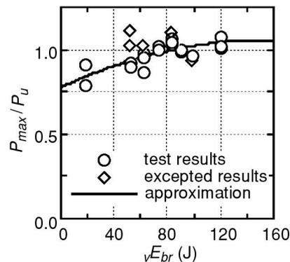
**Figure A3.5: Joint strength vs. fracture toughness relationships**
