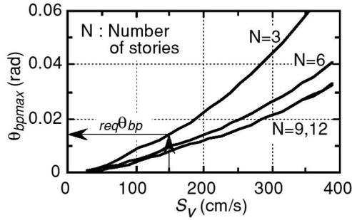
Figure 1: Required rotation angle of beam vs. pseudo-velocity of earthquake motion
