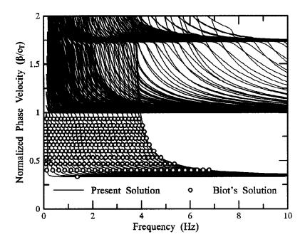
Fig. 2 Dispersion Curves of the Normal Modes
