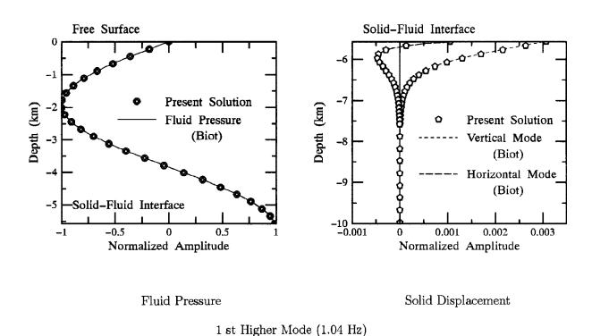
Fig. 3 Modal Shapes for Solid-Fluid Interaction System
