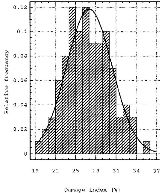
Fig. 5. Normal damage distribution.  $I_v \in [35-45]$ ,  $I_{MSK} = VIII$ , for concrete flat-slab buildings.
