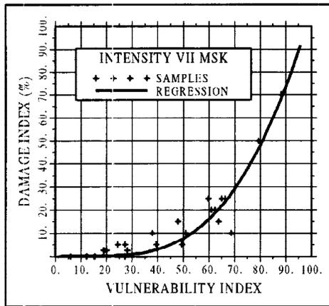
Fig. 1. Observed vulnerability function for masonry buildings,  $I_{MSK} = VII$ .
