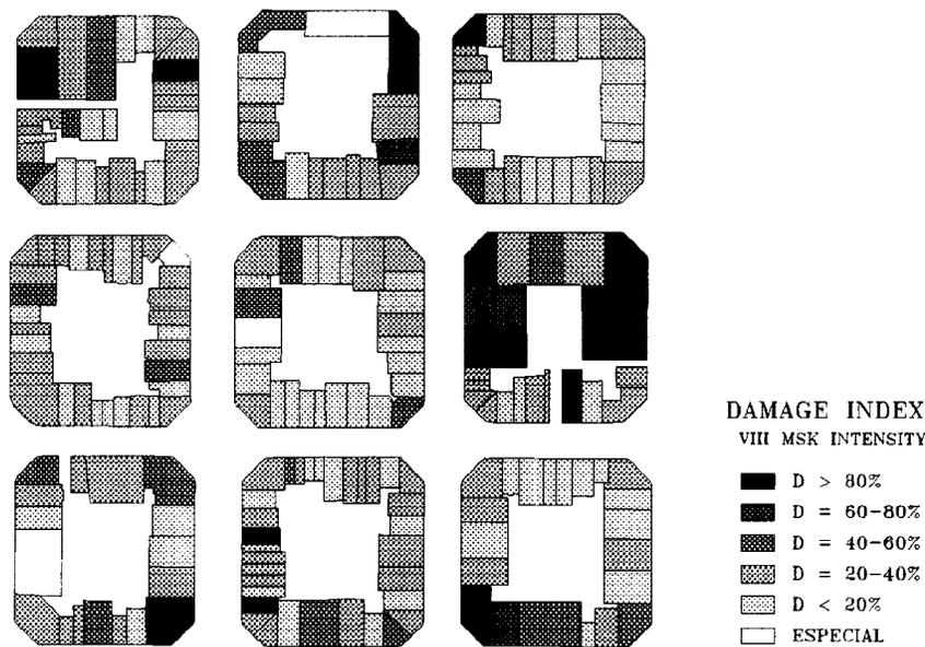
Fig. 10. Damage scenario for an earthquake of VIII MSK intensity level.
