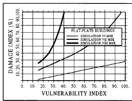
Fig. 8. Vulnerability functions obtained by simulation, for flat-slab buildings.
