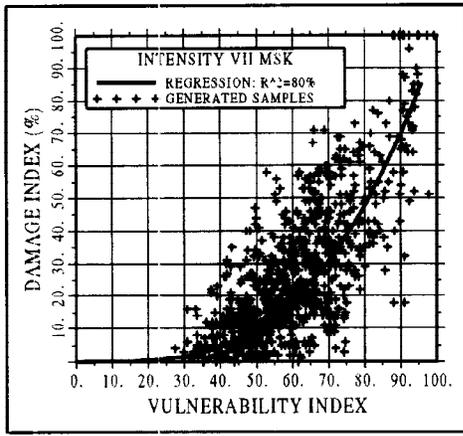
Fig. 3. Final building simulation and polynomial regression,  $I_{MSK} = VII$ .
