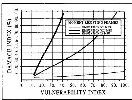
Fig. 7. Vulnerability functions obtained by simulation, for moment resisting frames.
