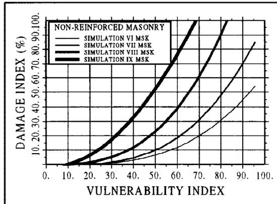
Fig. 6. Vulnerability functions obtained by simulation, for masonry buildings.
