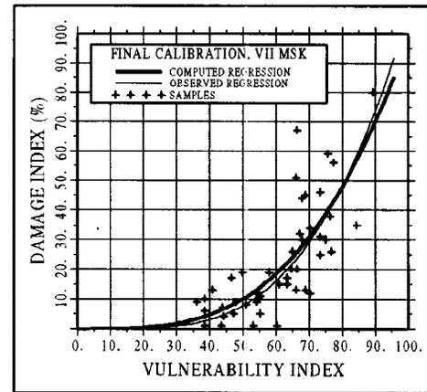
Fig. 2. Building simulation,  $I_{MSK} = VII$ , and comparison with the observed function.
