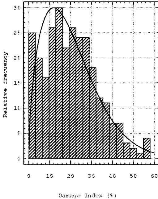
Fig. 4. Lognormal damage distribution.  $I_v \in [45,60]$ ,  $I_{MSK} = VII$ , for non-reinforced masonry buildings.
