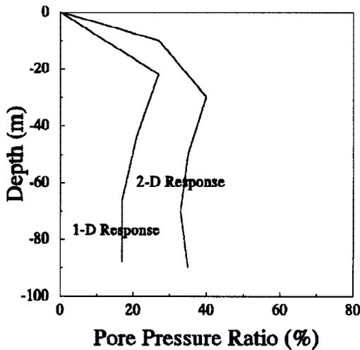
Fig.3 Peak Liquefaction response comparison for 1-D and wide 2-D valley
