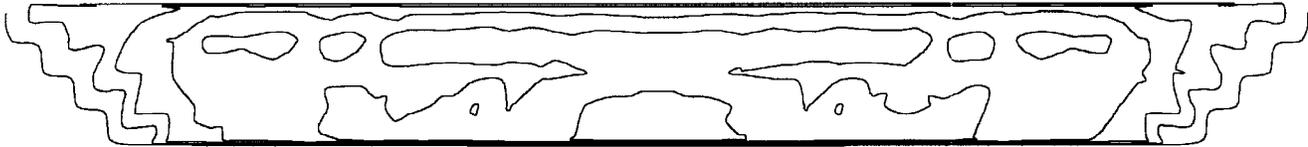
(b) 8:1 aspect ratio (Peak pore pressure ratio=0.5)
