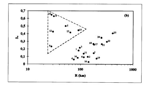
Fig. 1 Directivity of horizontal ground motion in the March 3, 1985 Central Chile earthquake versus hypocentral distance. (Dashed lines enclose all coastal stations in the macroseismic area). (a) Directivity for ground acceleration; (b) Directivity for ground velocity.
