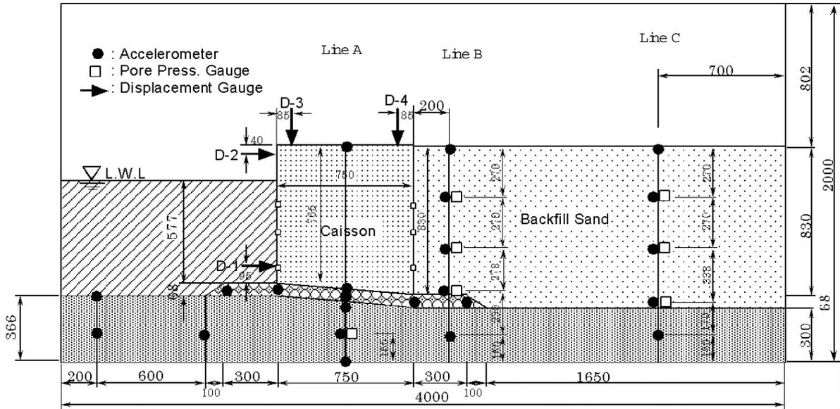
**Fig.2: Side view and measurement instrumentation in Case A3**
