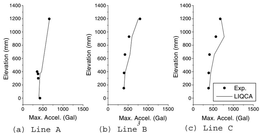
**Fig.4: Measured and calculated maximum acceleration (Case A3: 400 Gal)**
