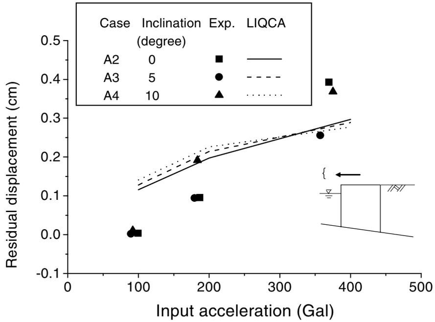
(a) Residual displacement at the bottom of the caisson
