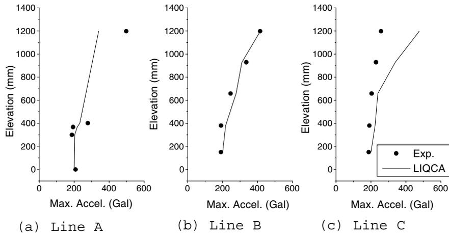
**Fig.3: Measured and calculated maximum acceleration (Case A3: 200 Gal)**
