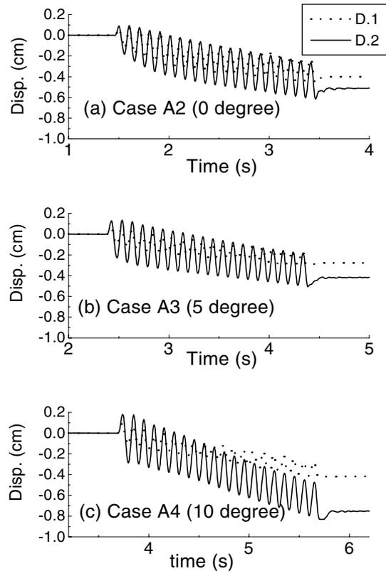
**Fig.5: Lateral displacements of caisson from tests (Input = 400 Gal: - sign indicates disp. towards sea)**
