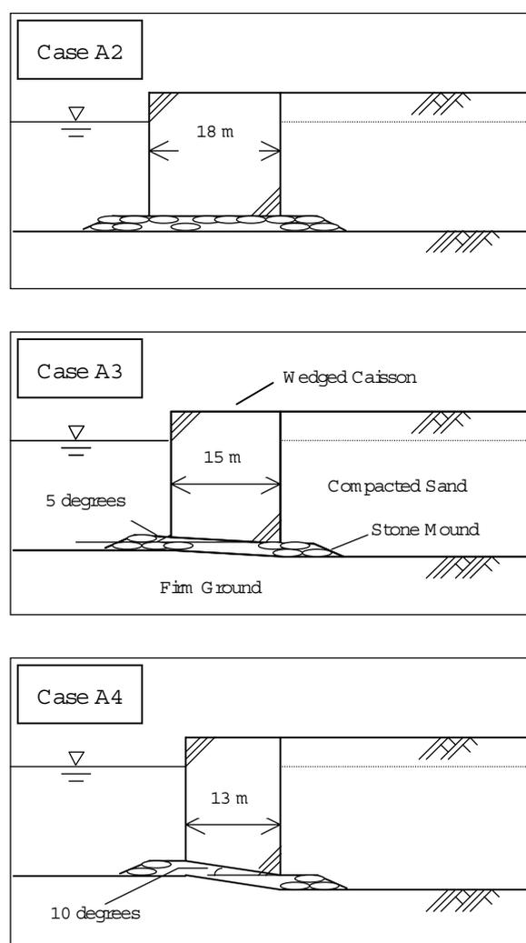
**Fig.1: Cross sections of test models.**
