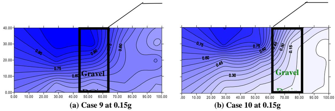
Fig 4: Contours of excess pore water pressure ratios
