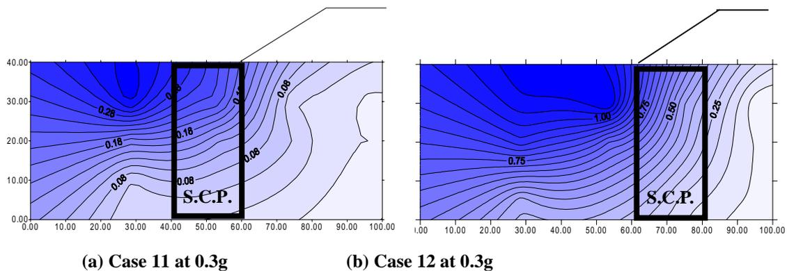
Fig. 5 Contours of excess pore water pressure ratios
