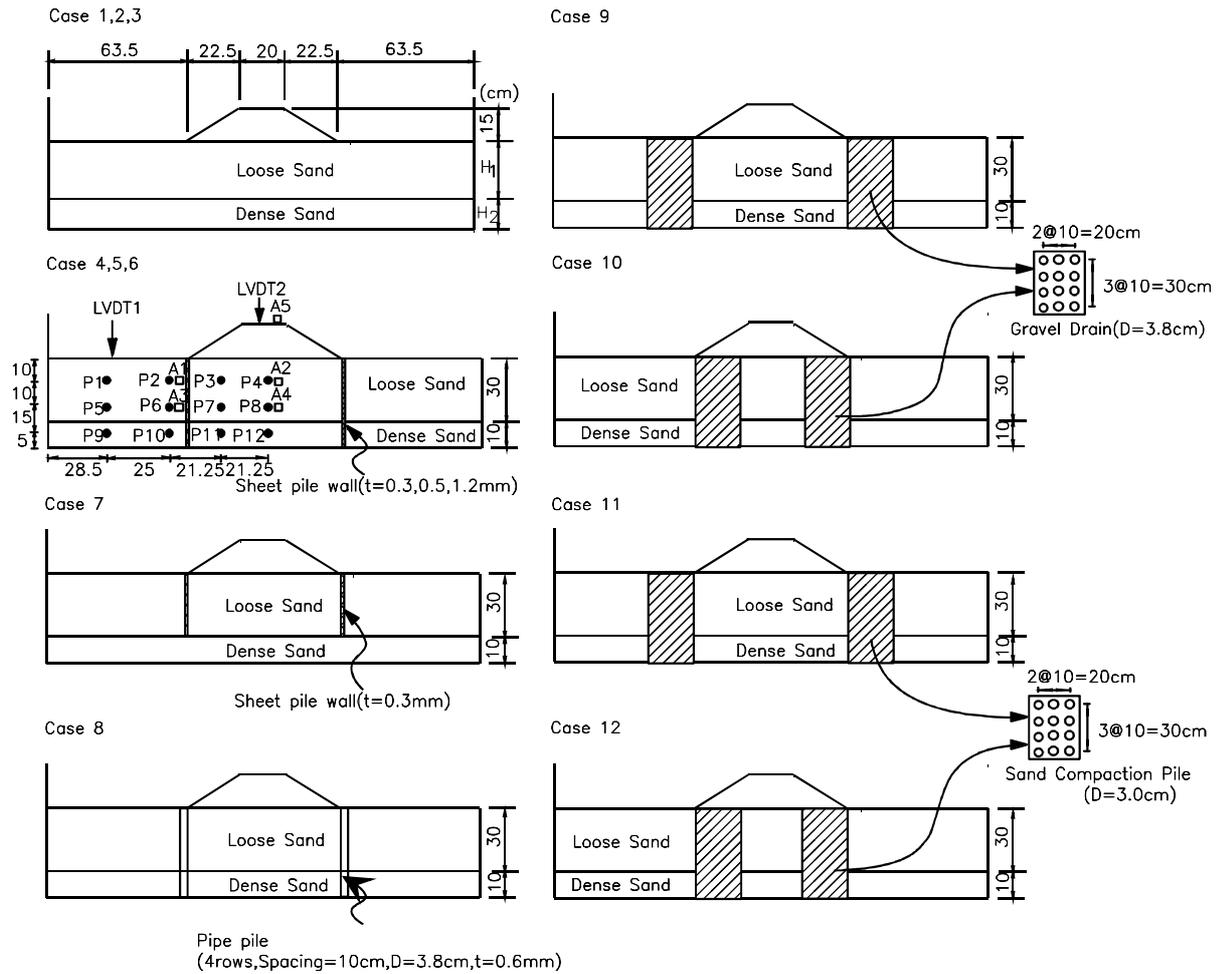
**Fig 1: Schematic drawings of each test set-up**
