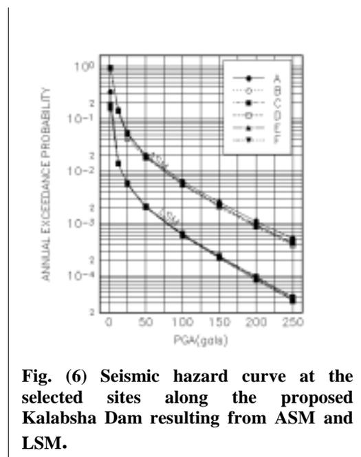
**Fig. (6) Seismic hazard curve at the selected sites along the proposed Kalabsha Dam resulting from ASM and LSM.**
