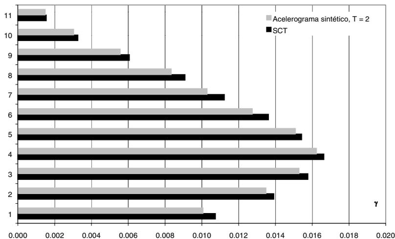
Figure 7 Interstorey drift obtained for the synthetic and for the actual accelerogram
