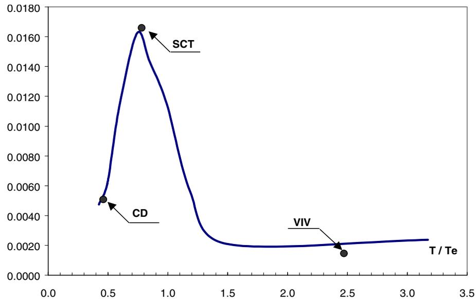
**Figure 8 Interstorey drift obtained for the synthetic and for three actual accelerograms.  $T=1.48$  sec is the period of the structure and  $T_e$  is the site dominant period**
