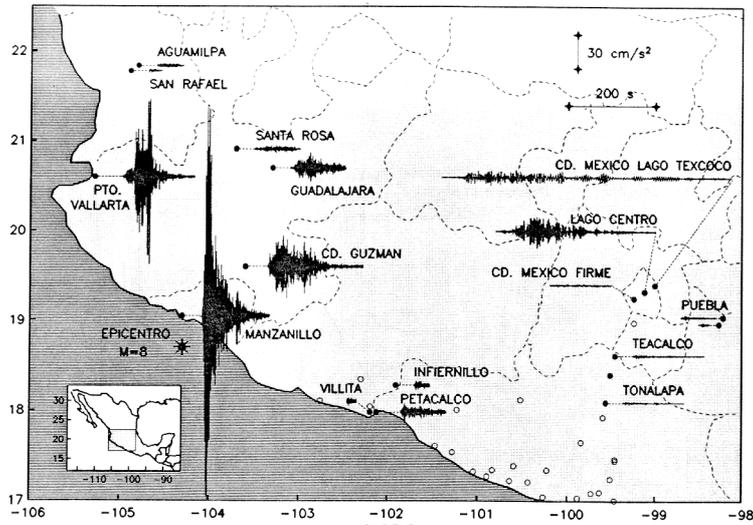
**Figure 2 Accelerations recorded along central Mexico during the 1995 earthquake**
