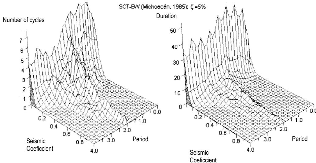
**Figure 5 Three-dimensional response spectra for site SCT during the 1985 earthquake: Number of cycles (left) and inelastic duration (right)**
