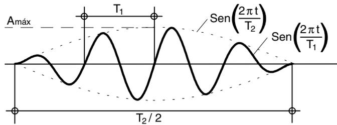
Figure 6 Synthetic accelerogram built with peak acceleration, duration ( $T_2/2$ ) and soil period ( $T_1$ )
