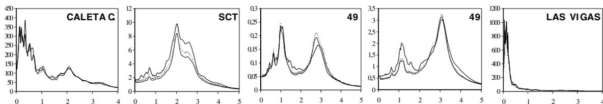
**Figure 4** Comparison of response spectra for different earthquakes, epicentral distances and soil conditions. Dark line: exact spectra; discontinuous line: RVT and computed duration; dotted line: RVT and duration given by equation 1
