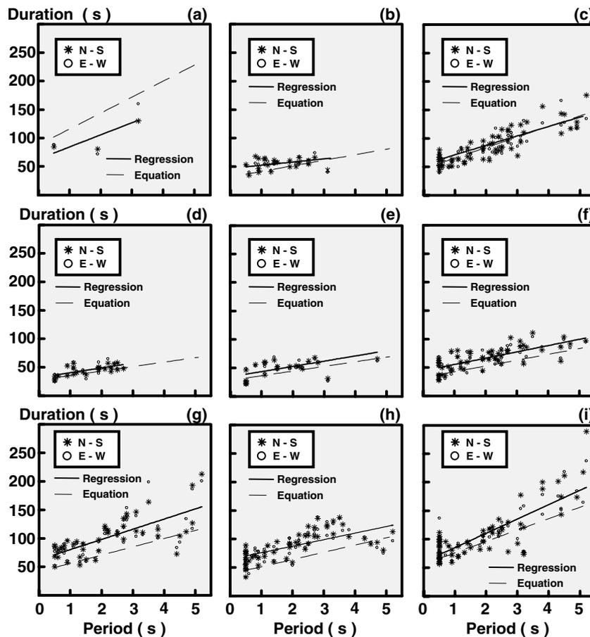
**Figure 3** Computed duration (symbols), regression for each earthquake and computed trend with equation 1. Earthquakes: a) 19/09/85, 8.1; b) 08/02/88, 5.7; c) 25/04/89, 6.9; d) 02/05/89, 5.2; e) 11/05/90, 5.3; f) 31/05/90, 5.8; g) 24/10/93, 6.6; h) 10/12/94, 6.3; i) 14/09/95, 7.3
