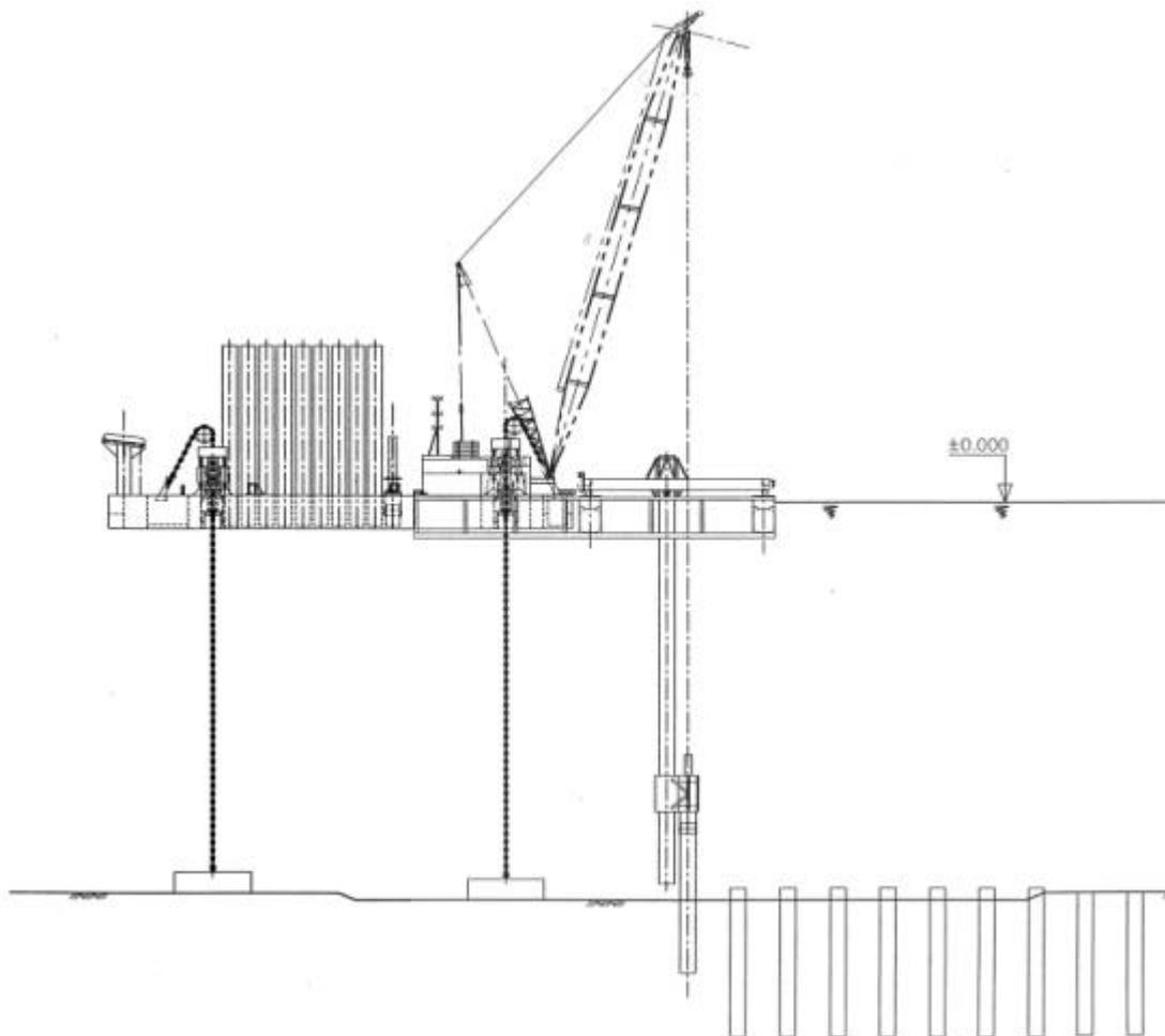
**Figure 6: Tension-leg barge**
