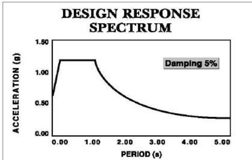
Figure 1: Design horizontal spectrum
