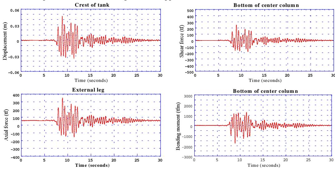
**Figure 6: Results of dynamic analyses (after retrofit)**
