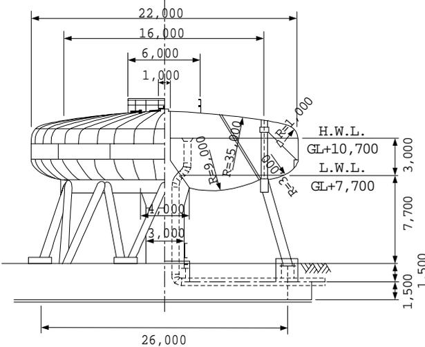
**Figure 1: Elevated steel water tank to be reviewed**
