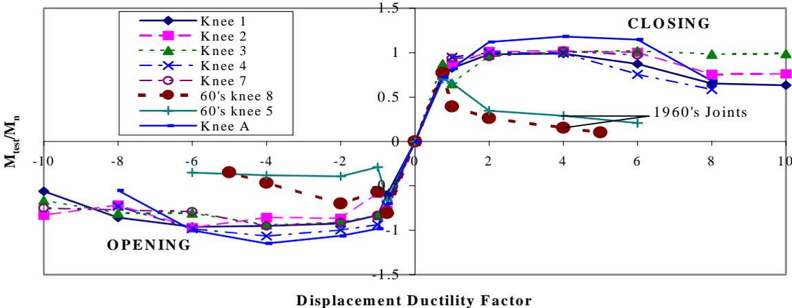
Figure 2: Applied Moment / Nominal Moment envelope for conventionally reinforced knee joints, including the two 1960's joints.
