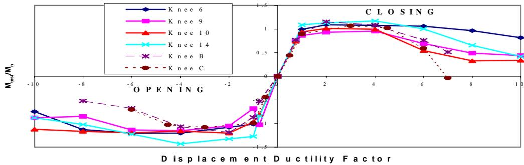
Figure 3:  $M_{test} / M_n$  for non-conventional knee joints with diagonal bars across re-entrant corner, except for Knee C with distributed beam bars (over beam depth).
