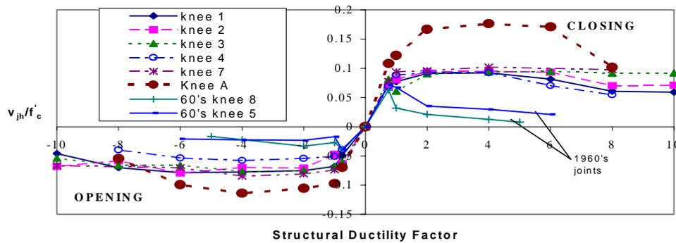
**Figure 4: Joint Shear Stress/ $f'_c$  versus Displacement Ductility for conventionally reinforced knee joints.**
