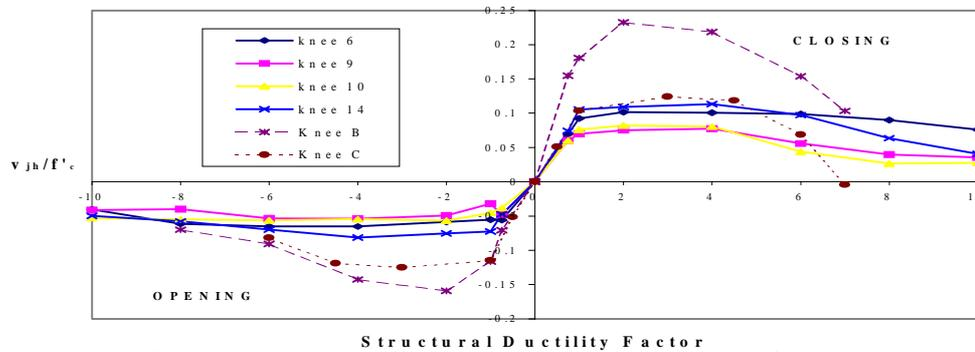
**Figure 5: Joint shear stress/ $f'_c$  against Ductility Factor for knee joints with extra diagonal bars across the re-entrant corner & knee C with distributed beam bars.**
