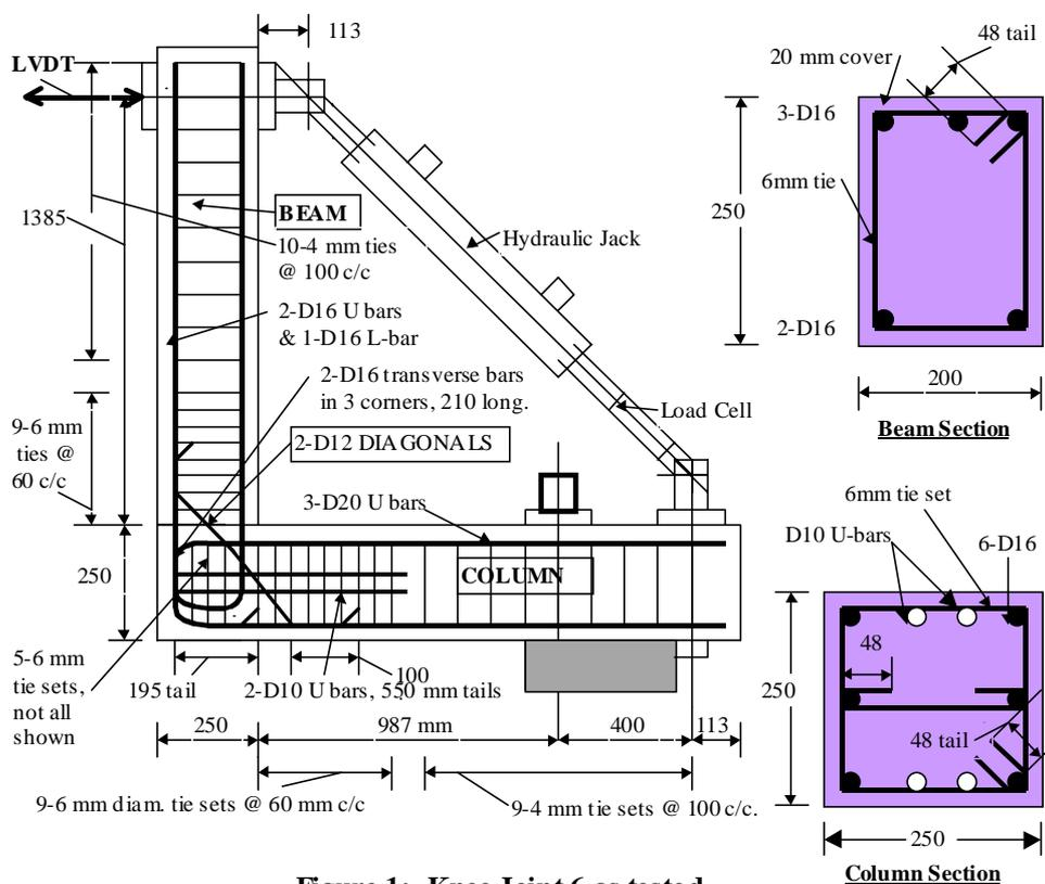
Figure 1: Knee Joint 6 as tested
