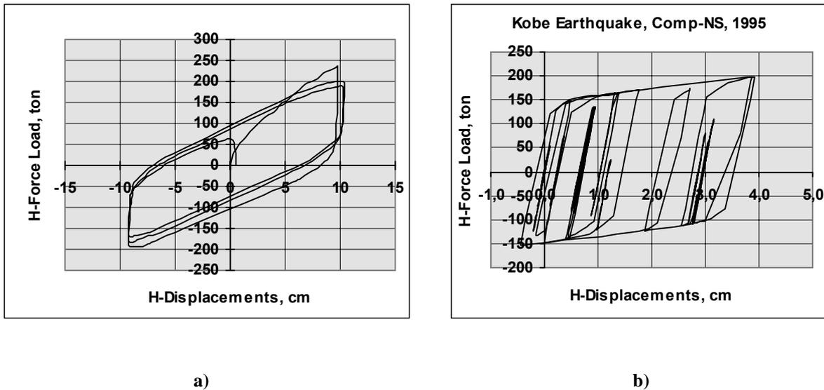
**Figure 5. Experimental (a) and computed (b) hysteretic characteristics of high-damping steel-rubber supports with lead cores**
