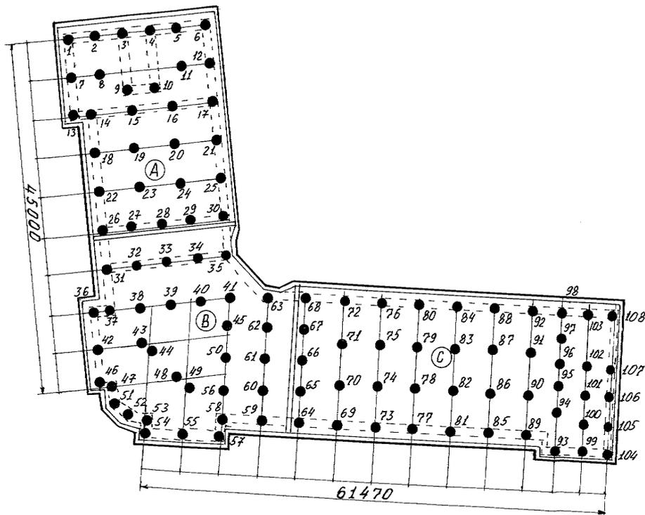
**Figure 3. Layout of isolators**
