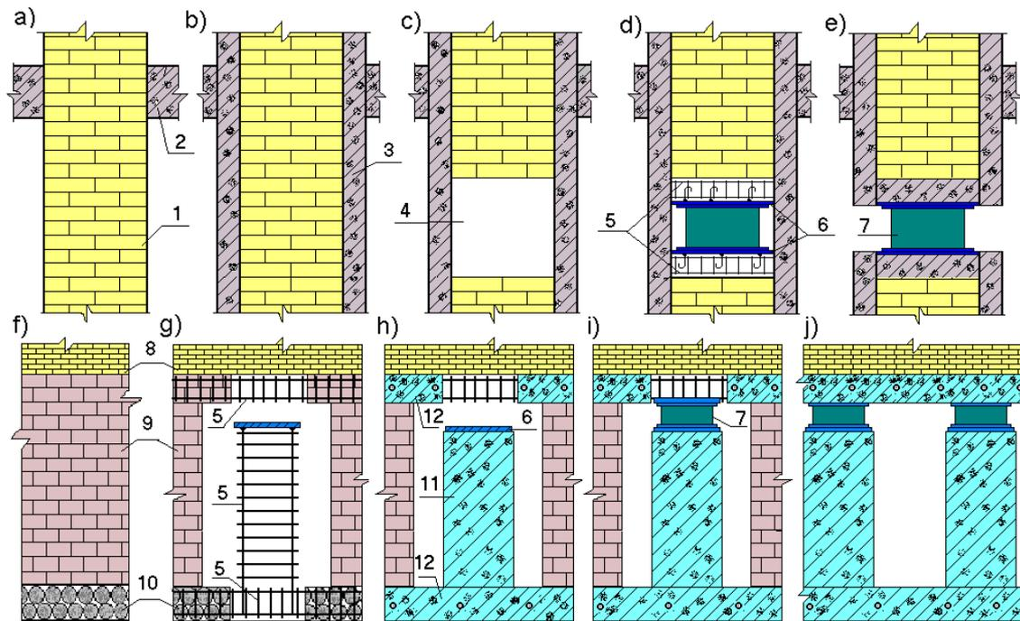
**Figure 4. Remodeling of the isolators installation procedure**
