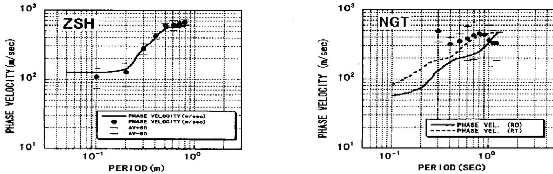
Figure 6. Comparison between theoretical and observed dispersion curve of phase velocity using the results of PS Logging Test and tripartite array observation of microtremors.
