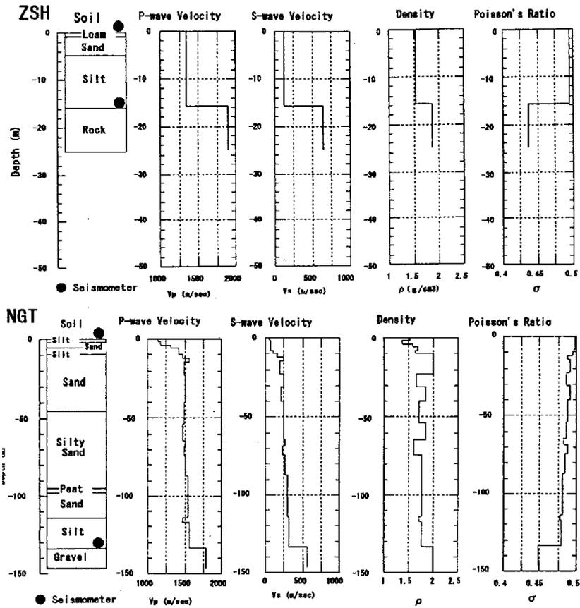
Figure 2. Soil profiles and results of PS Logging Test
