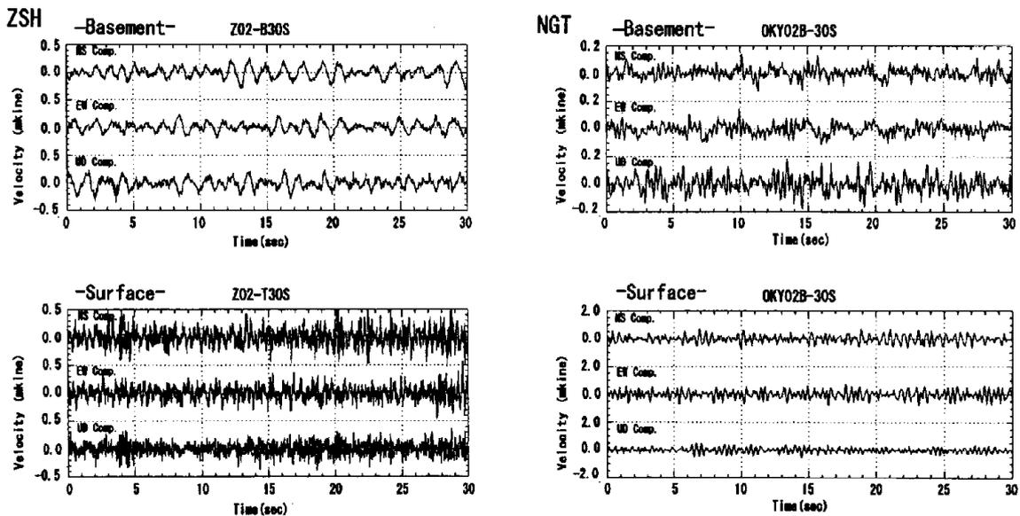
Figure 3. Examples of wave form microtremors observed at basement and surface simultaneously.
