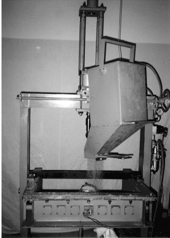
**Figure 5- the sand raining device and arrangement of the testing tank during preparation stage.**
