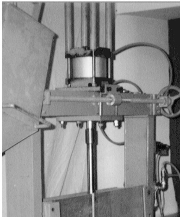
**Figure 2- the loading frame, the pneumatic cylinder, and its attachments to generate monotonic and cyclic loads.**
