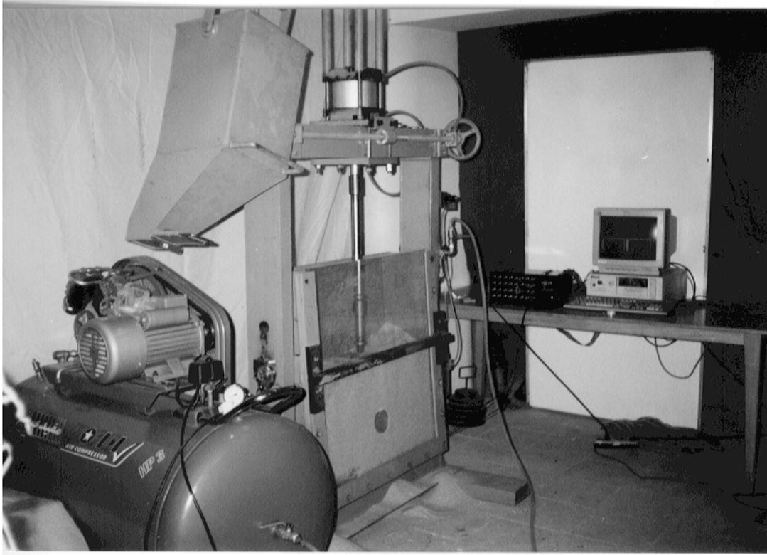
**Figure 1- the general view and main parts of the buried pipes testing system.**
