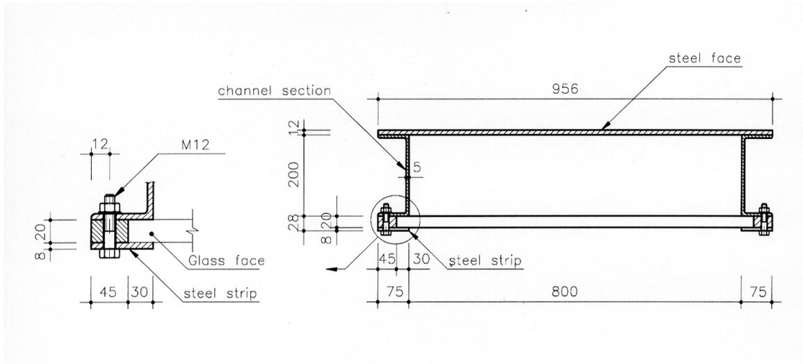
Figure 3- the horizontal section of the testing tank and details of fixing plexy glass. (dimensions in mm)
