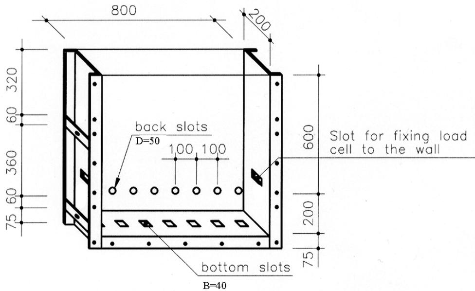
Figure 4- the position of the circular and square holes provided in the boundaries of the testing tank for setting transducers. (dimensions in mm)
