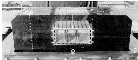
**Fig. 3 Model ground and model tunnel (three-span)**
