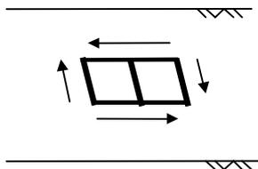
**Fig. 6 Direction of shear stresses on tunnel**
