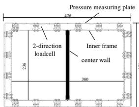
**Fig. 2 Model tunnel (two-span)**
