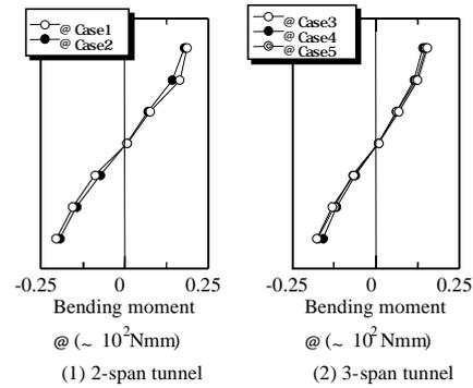
Fig. 9 Bending moment of center wall
