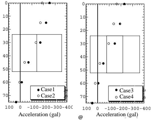
**Fig. 4 Response acceleration of ground far from the model tunnel**
