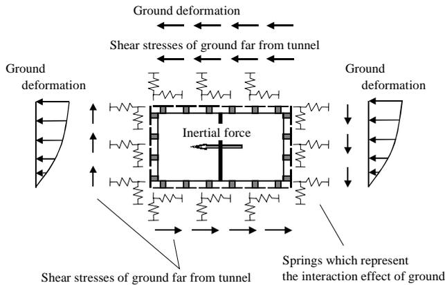
**Fig. 13 Concept of the seismic deformation method**
