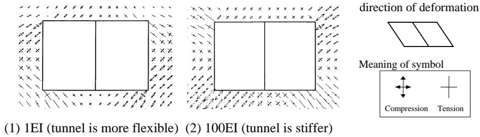
**Fig. 12 Principal stresses around the model tunnel**
