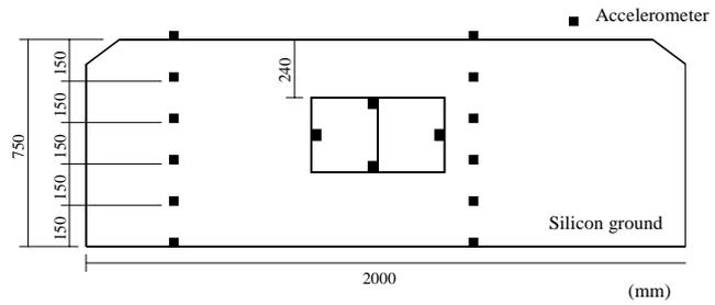
**Fig. 1 Model ground and accelerometers**
