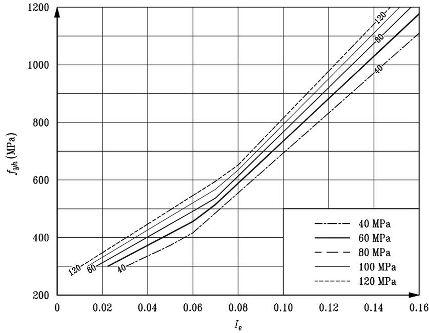
**Figure 3: Effective lateral steel yield strength as a function of concrete strength and effective confinement index**
