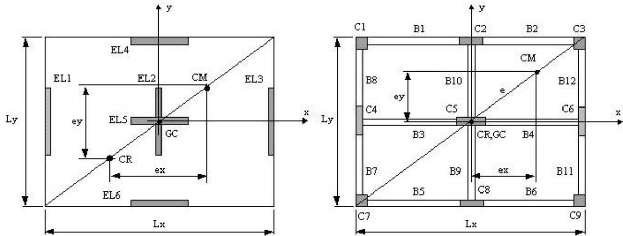
**Figure 1. Geometry of systems analyzed: (a) Shear-beam model (b) Reinforced concrete building**
