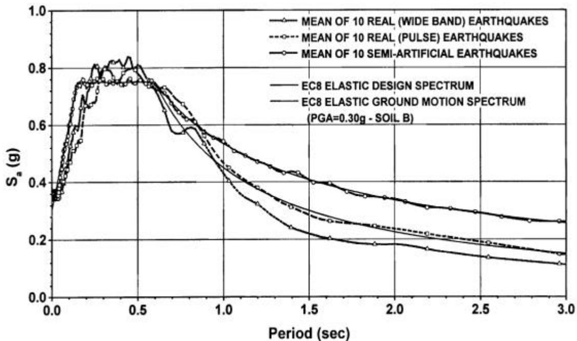
**Figure 2. Elastic design spectra and mean spectra of motions used**
