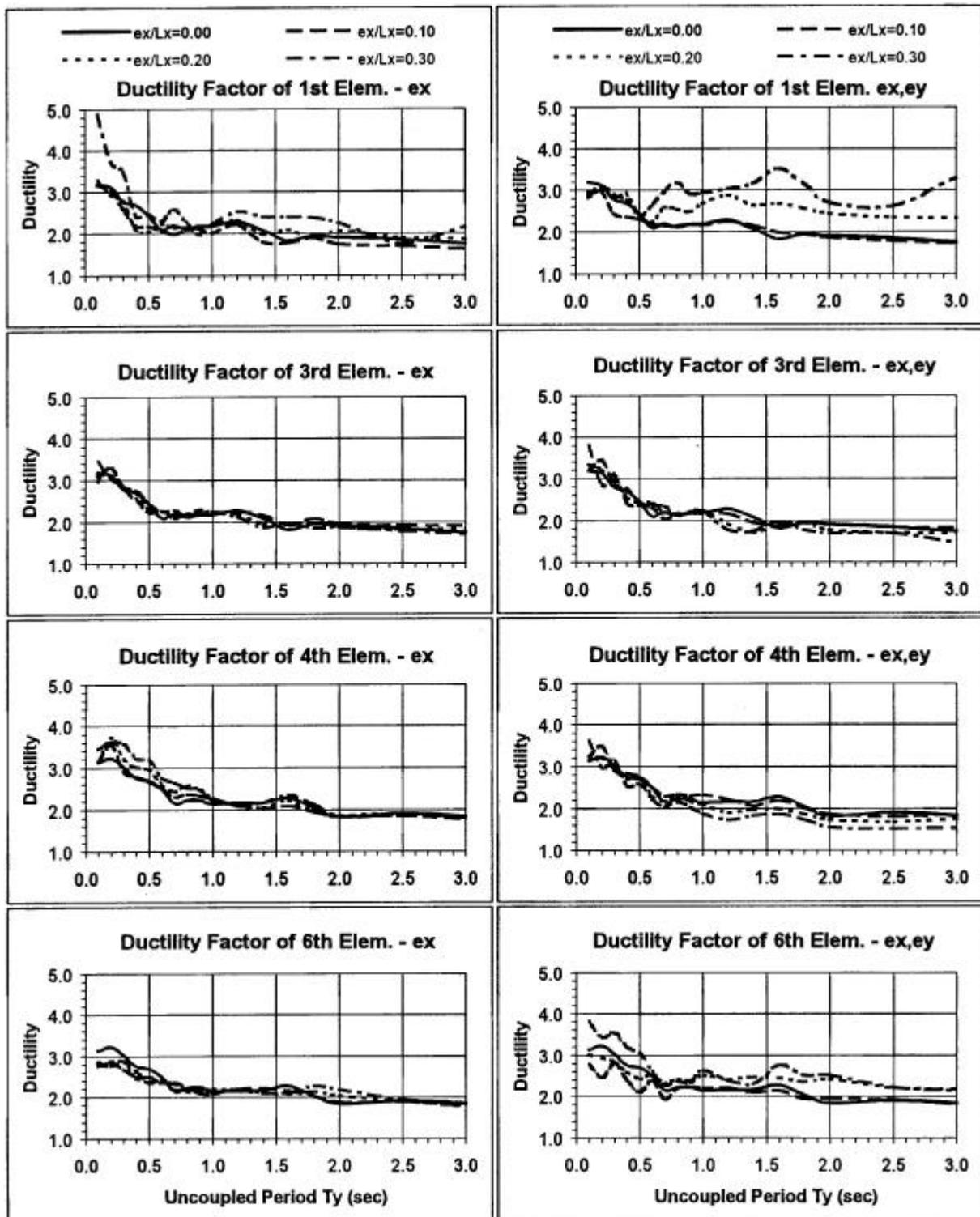
Figure 5. Results for mass eccentric systems with single and double eccentricity (motion group C)
