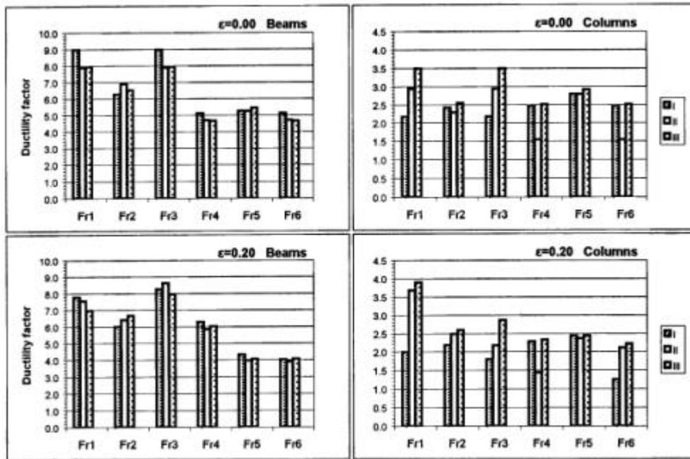
**Figure 6. Mean ductility demands of symmetric and mass eccentric ( $e=0.20$ ), one story, reinforced concrete buildings idealized with the plastic hinge model (design for three accidental eccentricities)**
