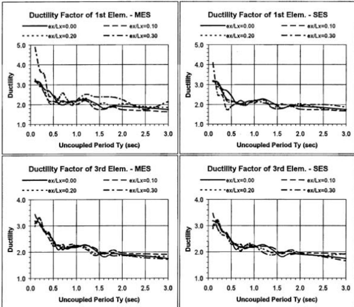
Figure 3. Comparisons of ductility demands between mass and stiffness eccentric systems (single eccentricity, motion group C)
