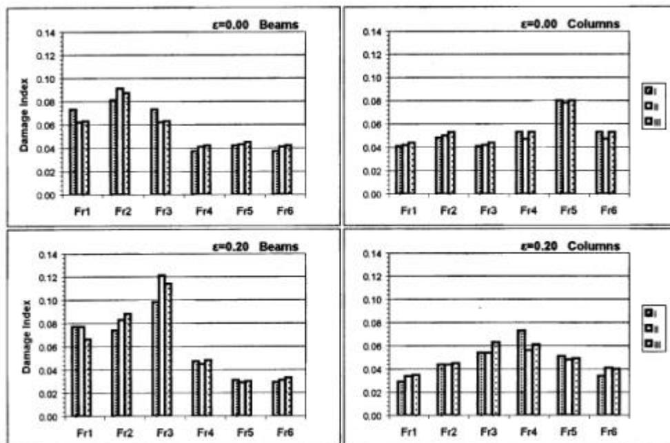
**Figure 7. Mean damage indices of symmetric and mass eccentric ( $e=0.20$ ), one story, reinforced concrete buildings idealized with the plastic hinge model (design for three accidental eccentricities)**
