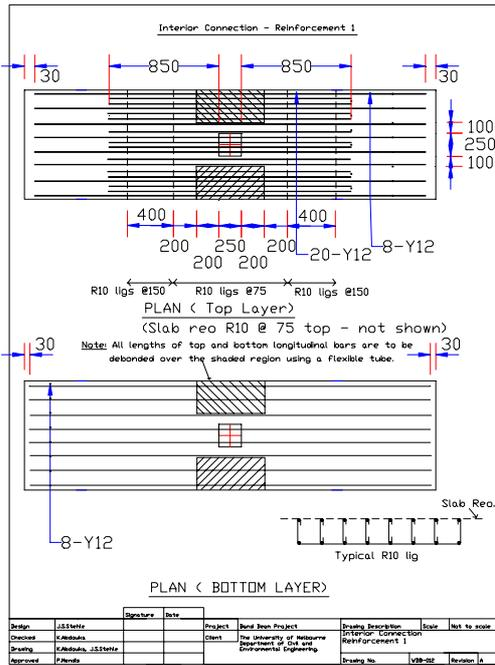
Figure 6: 2nd interior specimen beam detailing
