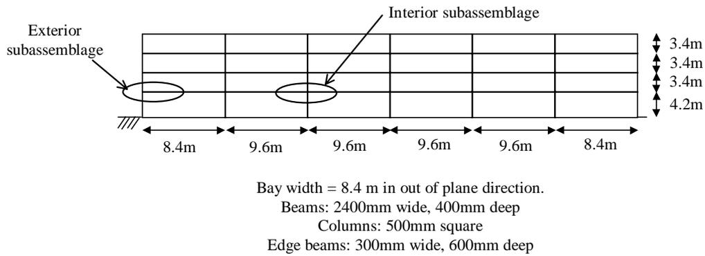
**Figure 1: Frame used in case study**
