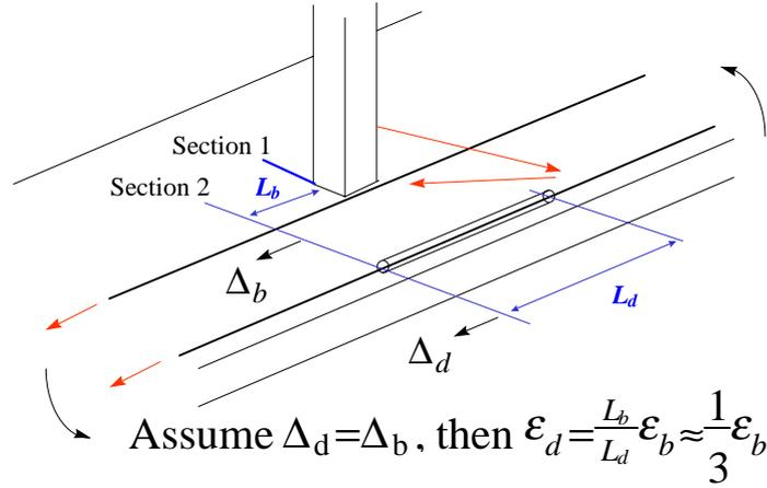
**Figure 9: Diagram showing the new load path due to debonding**
