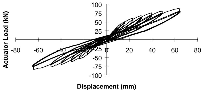
Figure 8: Hysteretic response of 2nd interior specimen
