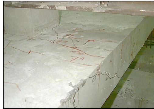
Figure 4: 1st interior specimen. Photo showing torsional cracking.
