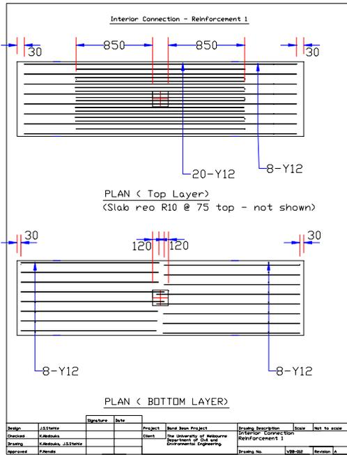
Figure 3: 1st interior specimen beam details
