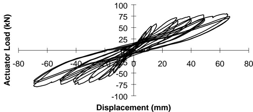
Figure 5: Hysteretic response of 1st interior specimen
