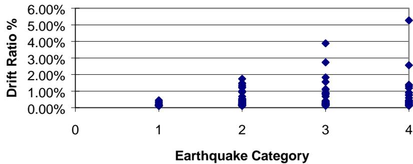
**Figure 11: Peak drift ratio response for 4 storey, 6 bay frame vs. earthquake category**
