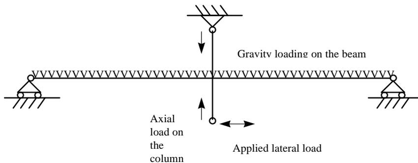
**Figure 2: Schematic diagram of test setup**
