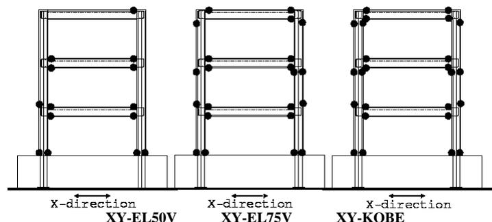
Figure 4: Locations of yielded main bars in X direction (Bidirectional tests)
