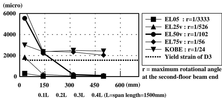
Figure 7: Maximum strain distributions of slab upper reinforcements at 2nd-floor (Unidirectional tests)
