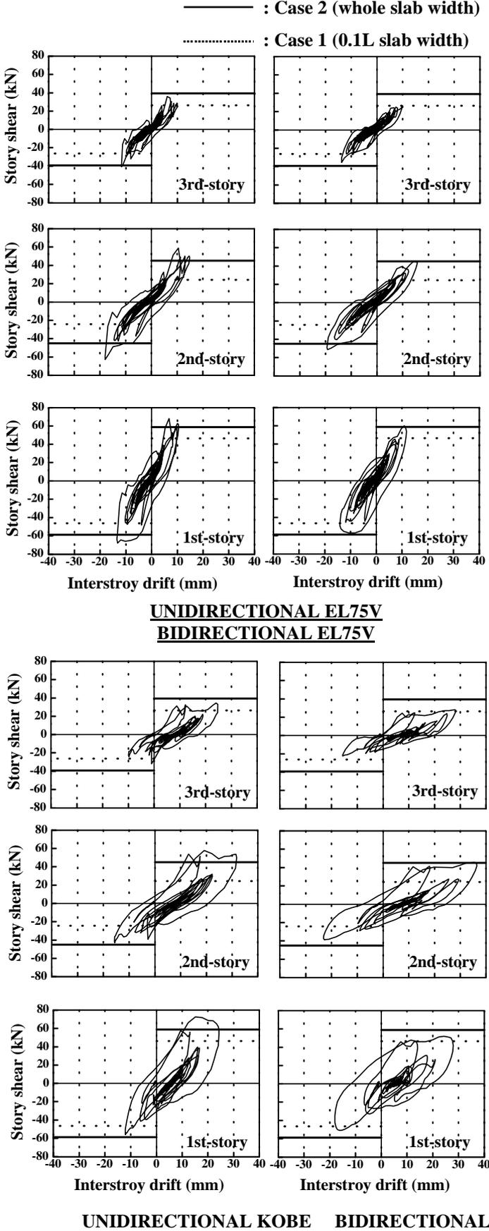
**Figure 5: Story shear-interstory displacement relations (Unidirectional tests vs. Bidirectional tests)**
