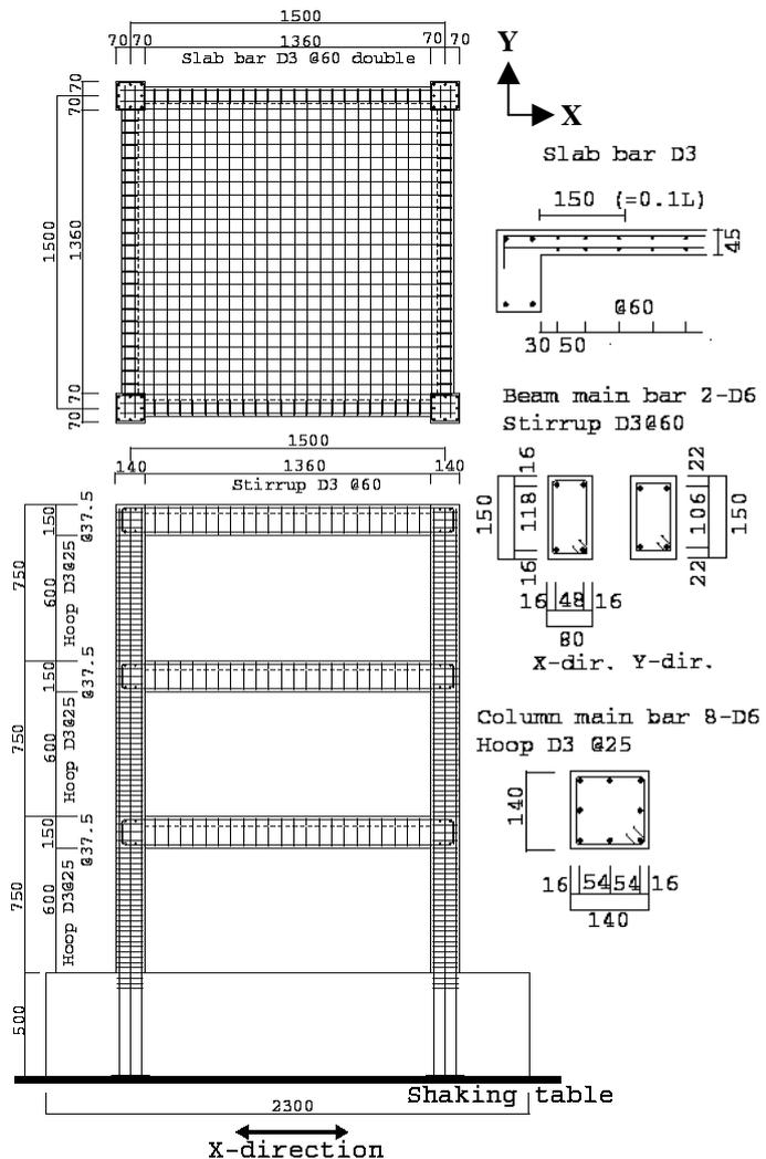
Figure 1: 1/4th-scale model test structure
