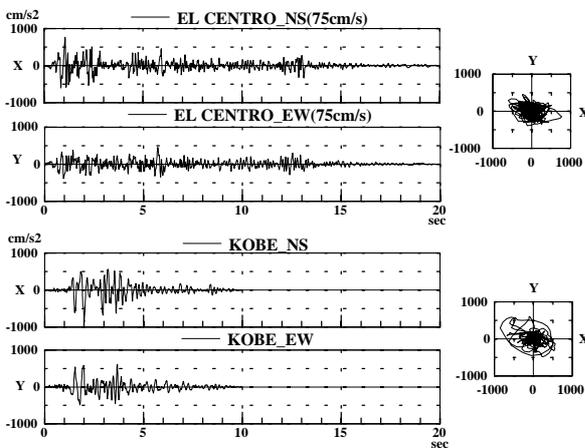
**Figure 2: Measured earthquake motions on the shaking table (El Centro at 75cm/s input level and Kobe of the bidirectional test)**
