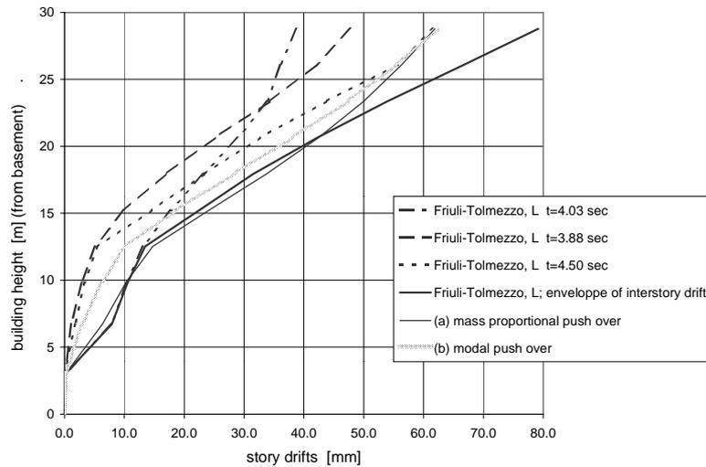
**Figure 8. Story drifts of the example building during "Friuli-Tolmezzo", longitudinal direction and in the push over analyses using different lateral force distribution**
