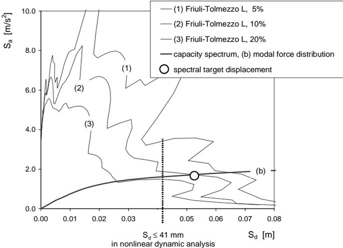
**Figure 6. Capacity spectrum method of the example building KJA for the earthquake Friuli-Tolmezzo, longitudinal direction. With the maximum spectral displacement in the nonlinear dynamic analysis, the equivalent damping is estimated to be 15%.**
