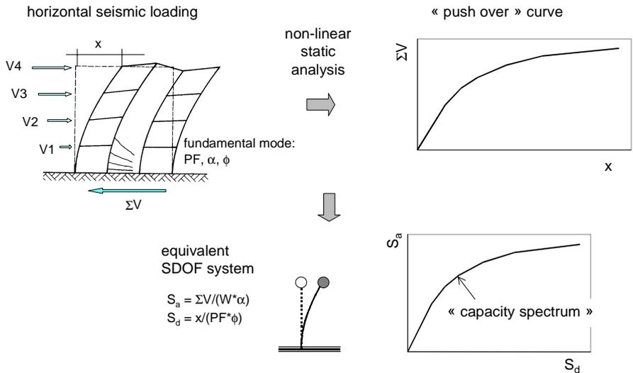
**Figure 1. The capacity spectrum as a result of the push over analysis**
