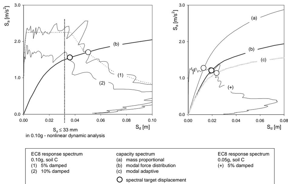
**Figure 5. The capacity spectrum method applied on the example building KJA, left for the 0.10g EC8 response spectrum and right for the 0.05g EC8 response spectrum, both for soft soil class C. On the left, additionally the maximum spectral displacement ( $S_d = 33$  mm) of the reference nonlinear dynamic analysis is given.**
