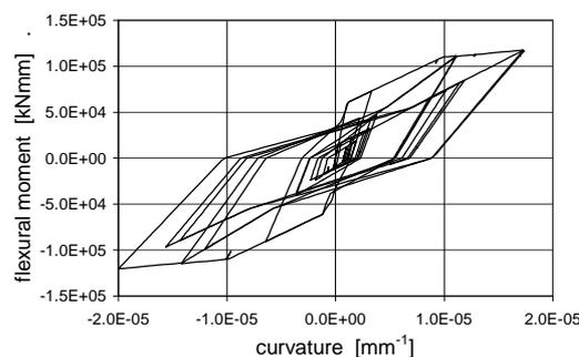
**Figure 3. Three-linear hysteretic model for the flexural behaviour of a r.c. wall implemented in Idarc2d [Valles, 1996 plus update version 5]**
