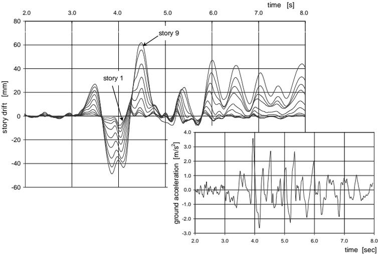
**Figure 7. Story drifts in the nonlinear dynamic analysis of the example building KJA during the earthquake timehistory Friuli-Tolmezzo, longitudinal direction, shown at bottom on the right.**
