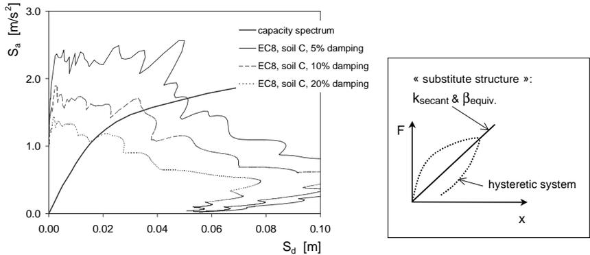
**Figure 2. Capacity spectrum method using the substitute structure approach**
