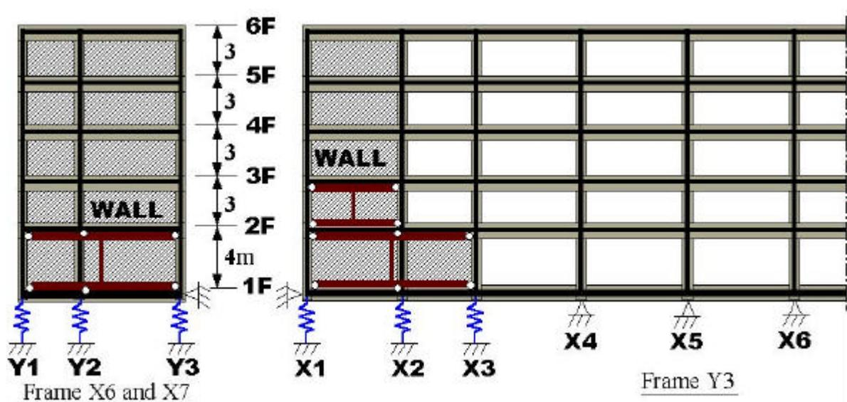
Figure 2: Frame elevation and frame models for the analysis
