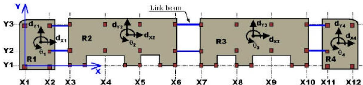
Figure 4: Multiple rigid diaphragms to represent the effect of segmented floor slabs
