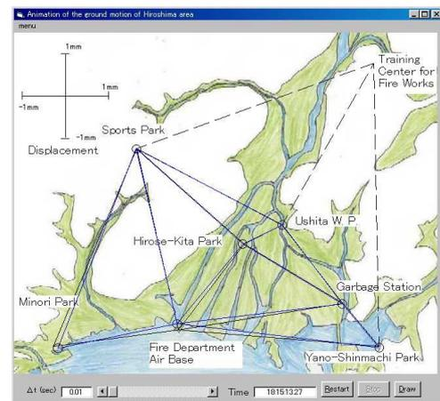
Fig. 13 Displacement distribution
