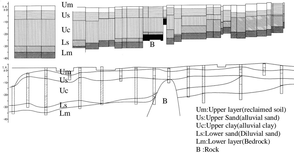
**Fig.7: Soil condition modeling**
