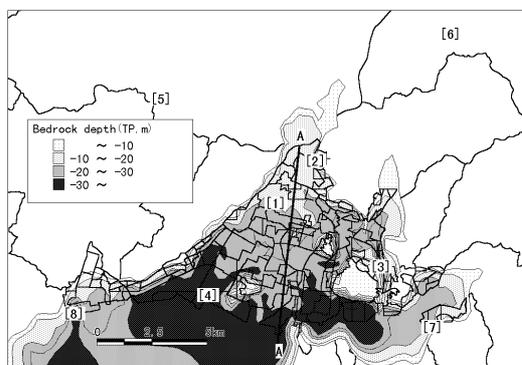
Figure 5: Bedrock depth and location of observation stations.
