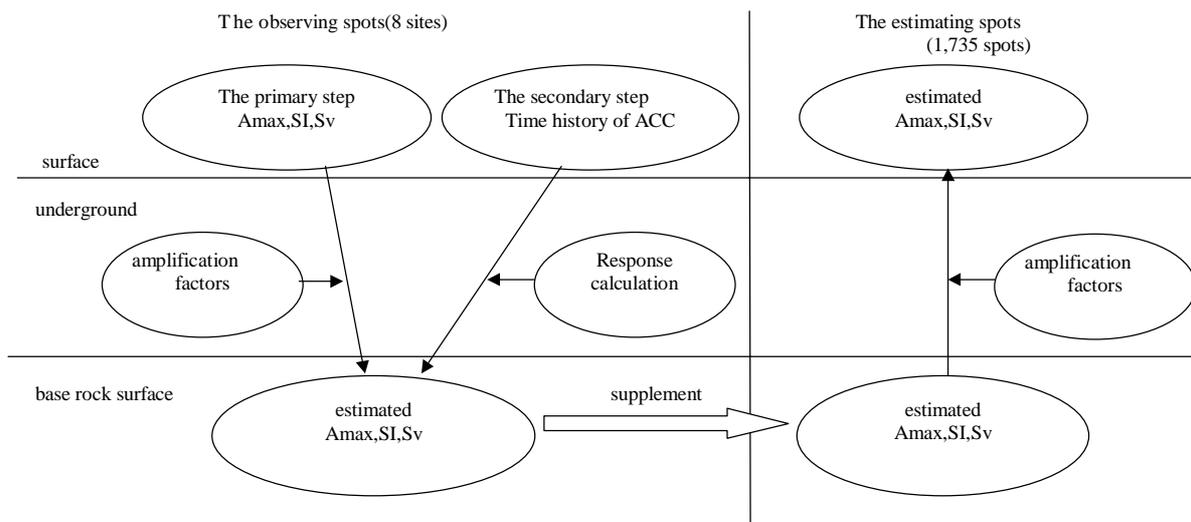
**Fig. 6: Flow of ground motion calculation**
