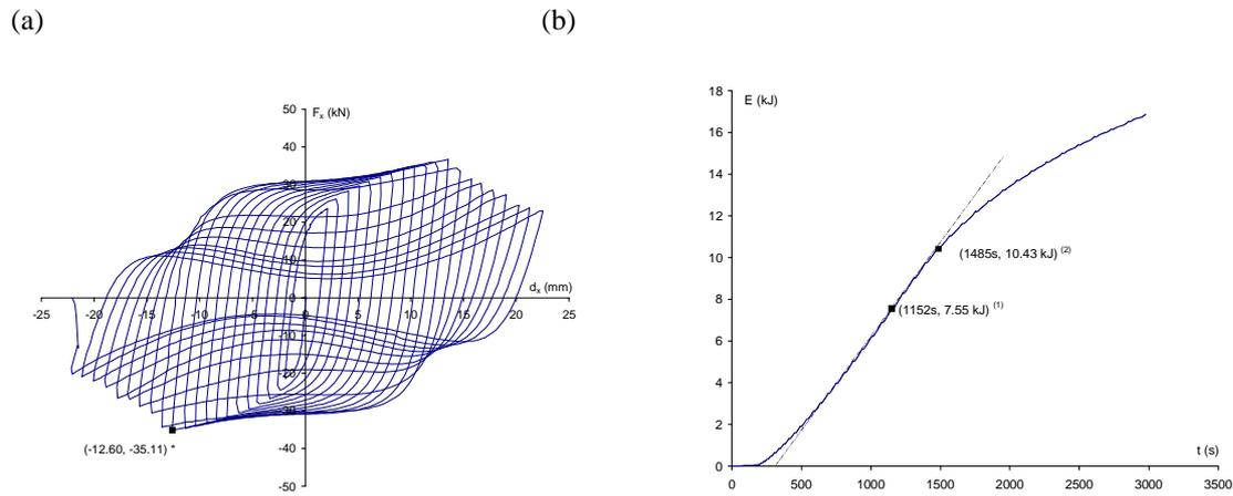
**Figure 3. (a) C-device load versus displacement hysteretic relationship (b) Evolution of the total dissipated energy of the ‘C’ specimen**
