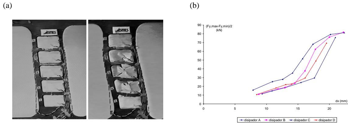
**Figure 4(a) A-device before an after web damage occurs. (b) Maximum cycle vertical force (semi-sum) versus displacement in the four devices**
