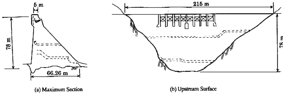
**Fig.7 The Maximum Section and Upstream Surface of a Real Dam**
