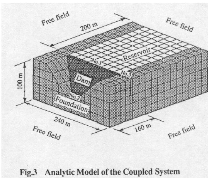
**Fig.3 Analytic Model of the Coupled System**
