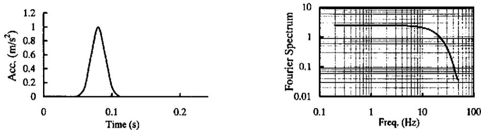
**Fig.4 Input Wave (Gauss Pulse)**
