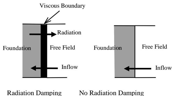
**Fig.1 Model for Evaluation of Radiation Damping of Dam – Foundation System**
