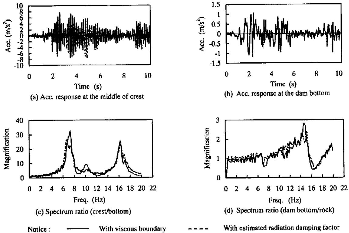
**Fig.8 Comparison between the Results Got with Viscous Boundary and Those Got with Radiation Damping Factor**
