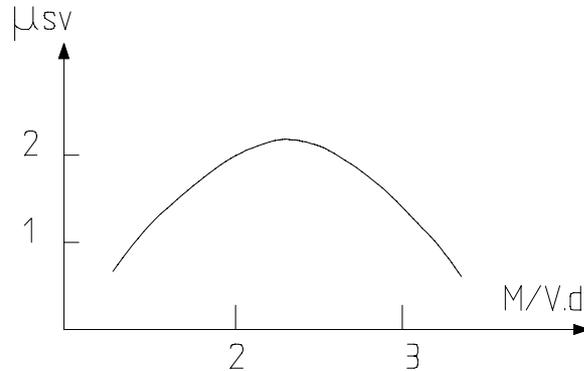
**Fig.10 Shear span vs. shear ductility**
