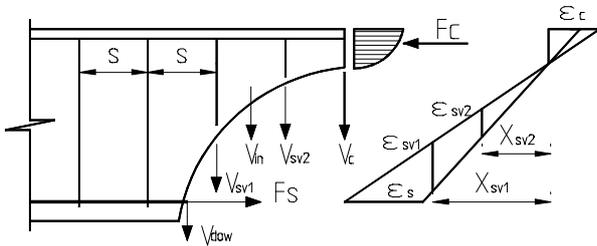
**Fig.7 Shear forces and strains distributions**
