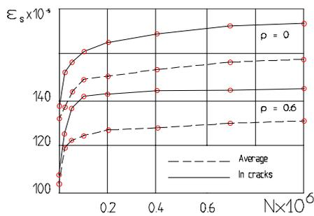
**Fig.5 Strains in longitudinal reinforcement**
