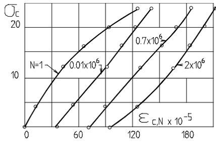
Fig.1 Stress-strain relationship for concrete
