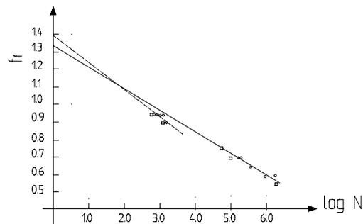
fig.4 fatigue of reinforcement
