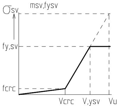
**Fig.9 Shear forces vs. stirrup stresses**
