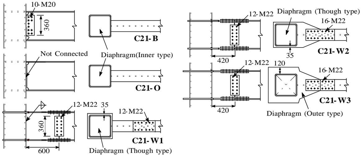
**Fig.2 Beam End Connection Details**
