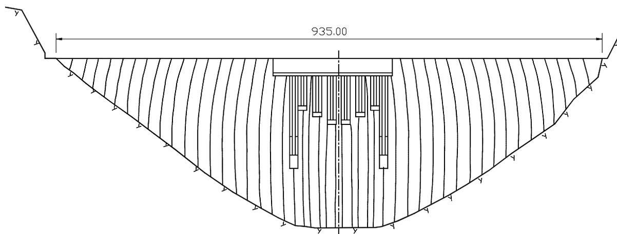
**Figure 1: Layout of contraction joints of the Xiaowan Arch Dam**
