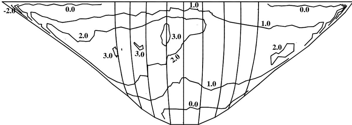
(d) Maximum stress of cantilever component on downstream face(with joints)
