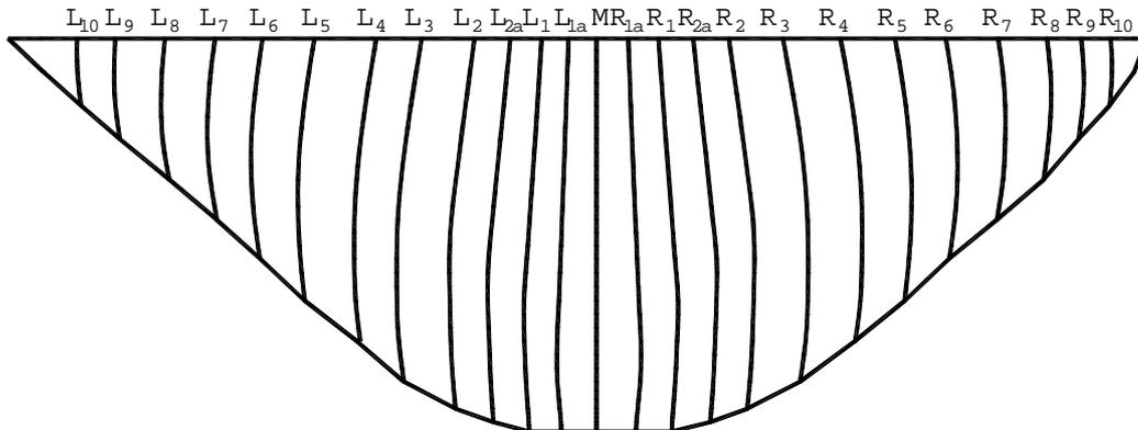
**Figure 4: Simulation of Contraction joints for Xiaowan Arch Dam (Case of 25 Joints)**
