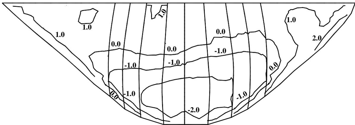
(b) Maximum stress of arch component on upstream face (with joints)
