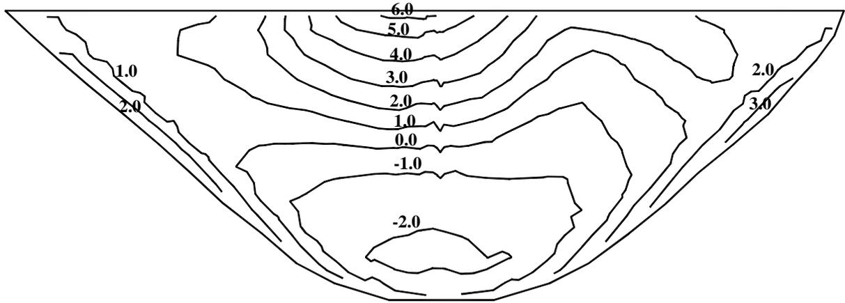
(a) Maximum stress of arch component on upstream face (without joints)
