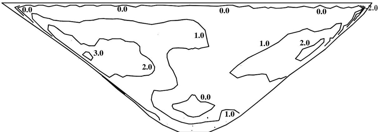
(c) Maximum stress of cantilever component on downstream face (without joints)
