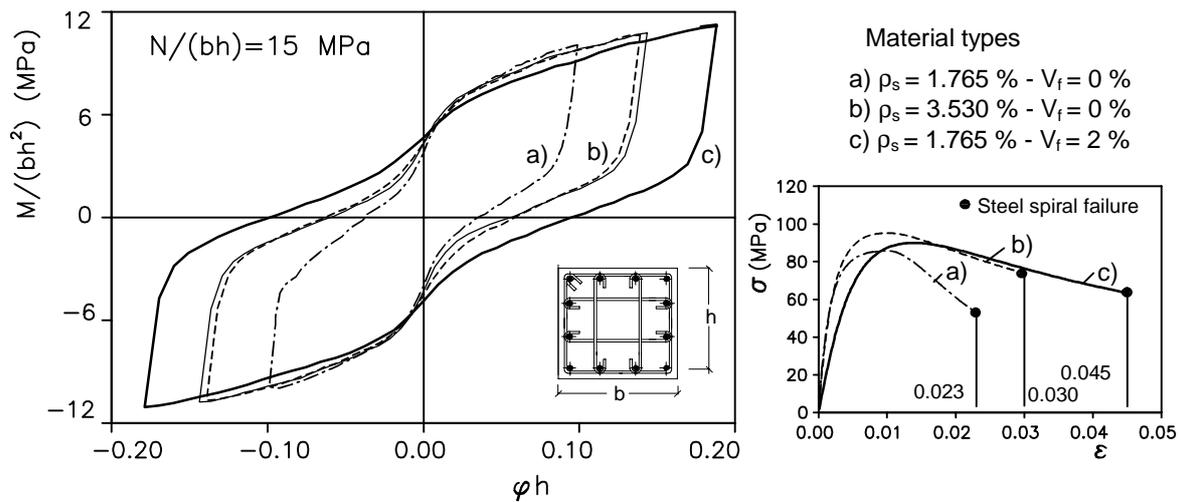
Figure 6:  $M/(bh^2) - \phi h$  curves with variation in the material type
