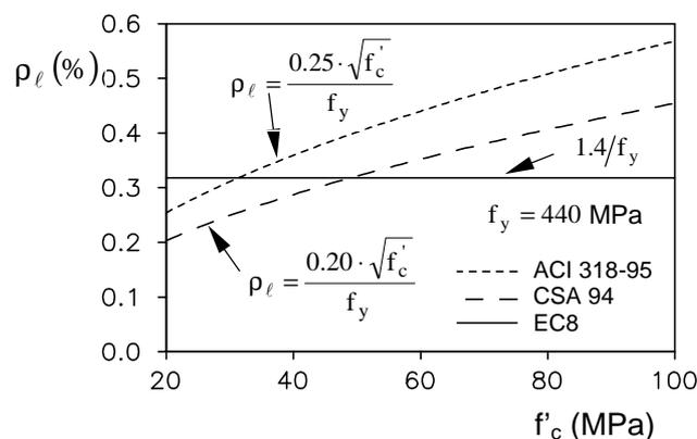
Figure 7: Minimum flexural reinforcement
