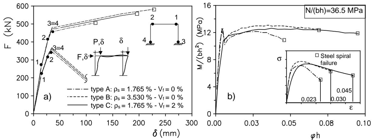
**Figure 9: Collapse mechanism for different confining levels : a) base shear-lateral displacement curves ; b) plastic hinges at column base sections**
