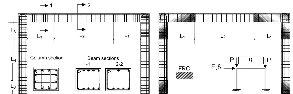
**Figure 8: Structural scheme**
