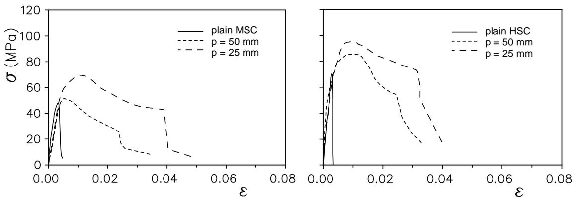
**Figure 2: Stress-strain curves of plain concrete ( $V_f = 0$ ) with steel spirals**
