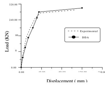
**Fig. 8 Comparison of DDA solutions with experimental results: Load-deflection relation of a RC frame partially filled with masonry wall**
