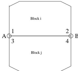
**Fig. 4 Two blocks just in contact at time  $t = 0$**
