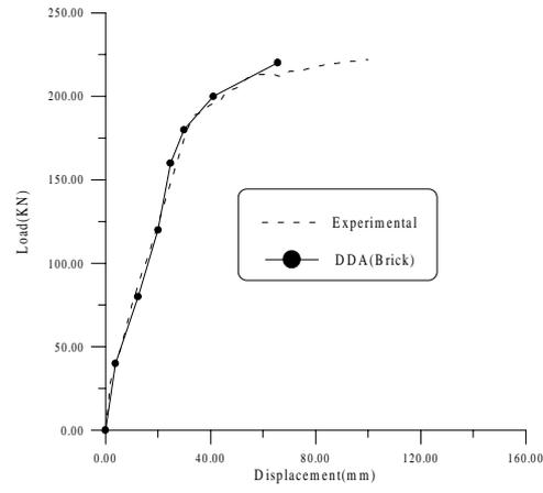
**Fig. 6 Comparison of DDA solutions with experimental results: Load-deflection relation of a RC frame**
