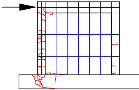
**Fig. 9 Failure configuration of RC frame completely filled with masonry wall (Experimental result)**
