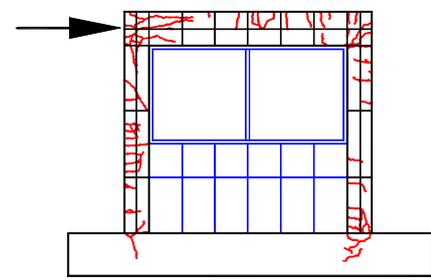
**Fig. 7 Failure configuration of RC frame partially filled with masonry wall (Experimental result)**
