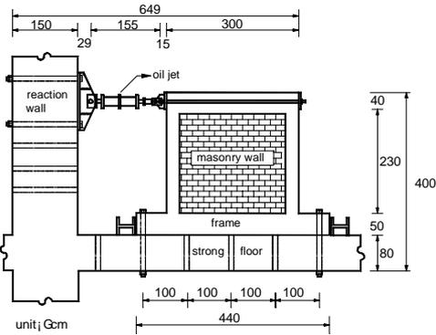
**Fig. 1 The experimental system**
