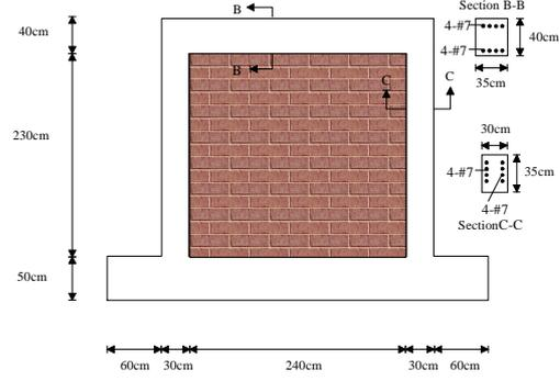
**Fig. 2c RC frame completely filled with masonry wall**
