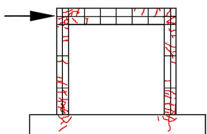
**Fig. 5 Failure configuration of RC frame (Experimental result)**
