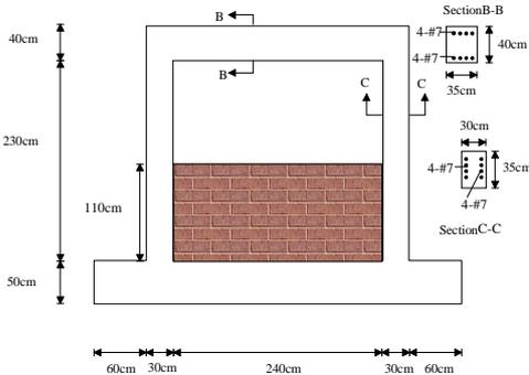
**Fig. 2b RC frame partially filled with masonry wall**
