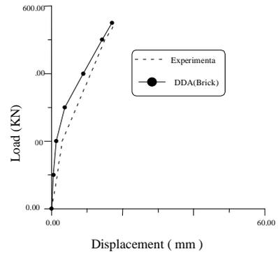
**Fig.10 Comparison of DDA solutions with experimental results: Load-deflection relation of a RC frame completely filled with masonry wall**
