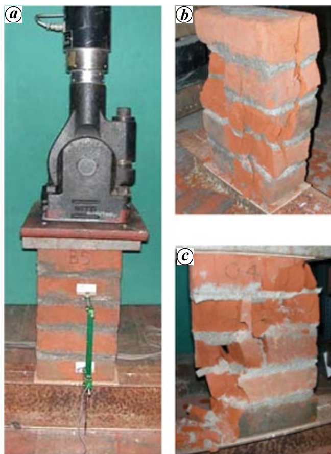
Figure 1. a, Test set-up for compression testing of masonry prism. b, c, Typical failure modes showing vertical splitting of specimens.
