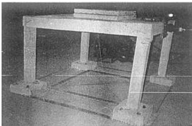
Fig 1 One-third scaled model of RC frame used in the experimental study (seismic model at a drift ratio of 6 percent)
