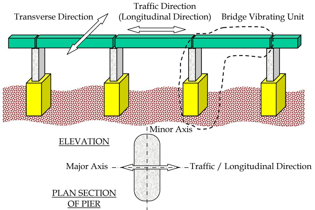
Figure 2: Single pier bridge vibration unit with typical orientation of the pier section.
