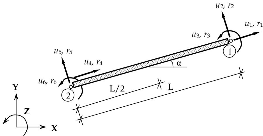
**Figure 8:** End-forces and displacement quantities on a segment in local coordinates.
