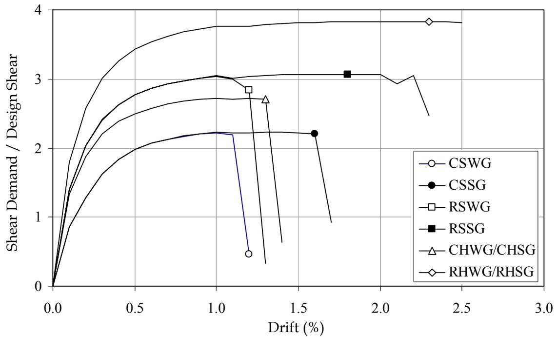
**Figure 11:** *Effect of Cross-Section Geometry:* Lateral load-deformation response of 5 m tall piers. Piers having solid circular and rectangular cross-sections and with design shear reinforcement have stable post-yield response.
