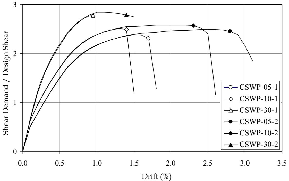
**Figure 13:** *Effect of Axial Load:* Lateral load deformation response of solid circular piers with axial load ratios of  $0.05f'_cA_g$ ,  $0.10f'_cA_g$  and  $0.30f'_cA_g$  with nominal and increased transverse reinforcement. Axial load increases overstrength shear demand while transverse reinforcement increases displacement ductility.
