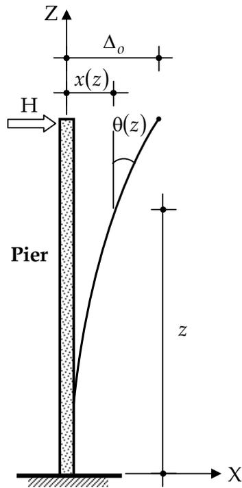
**Figure 7:** Initial lateral and rotational deformation of cantilever pier section for specified tip displacement.
