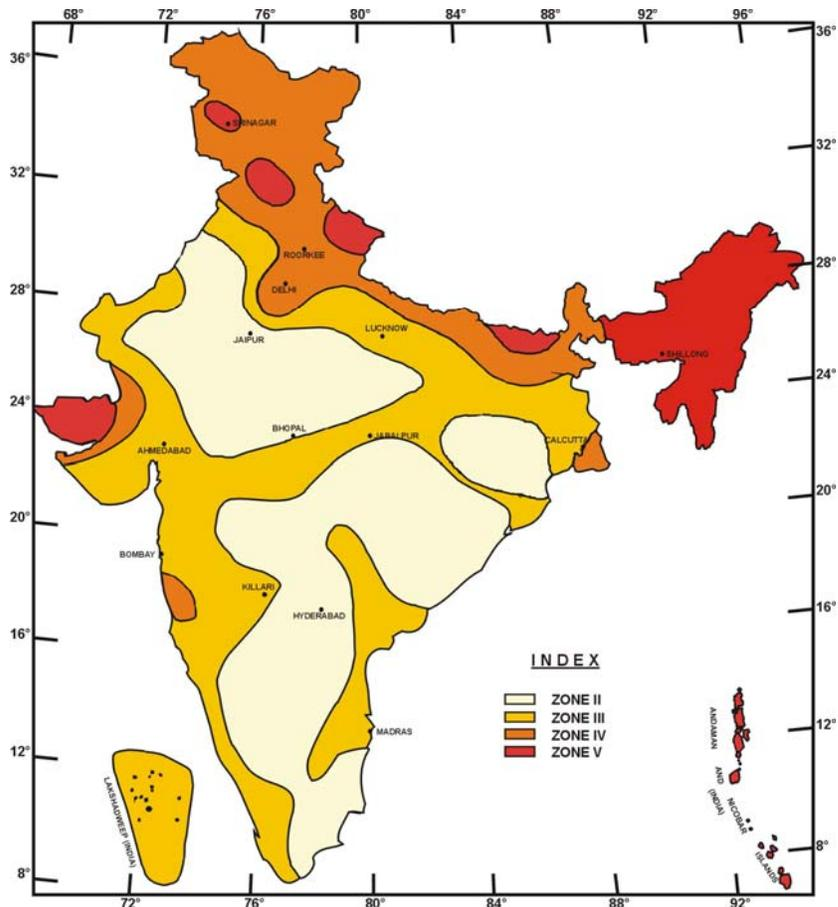
Figure 1: Seismic Zones and Zone Map of India [IS:1893 (Part 1), 2002].
