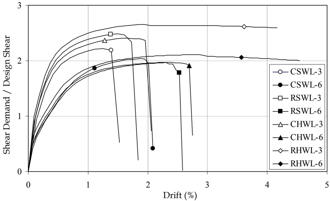
**Figure 12:** *Effect of Pier Slenderness:* Lateral load-deformation response of solid-circular, solid-rectangular, hollow-circular, and hollow-rectangular piers having slenderness ratios 3 and 6 with corresponding nominal shear capacities. Short piers with slenderness of 3 are vulnerable in shear.
