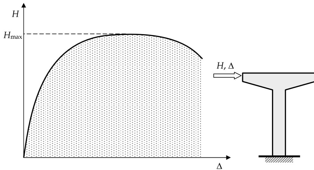
**Figure 10:** Maximum shear demand on the pier during the entire displacement loading history.
