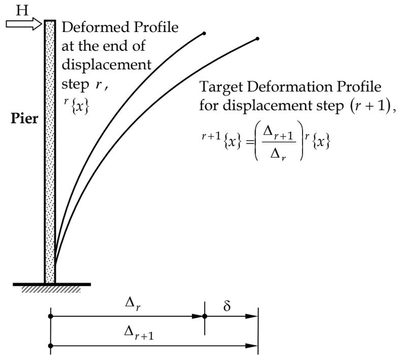
**Figure 9:** Target displacement profile of pier for next displacement step in pushover analysis.
