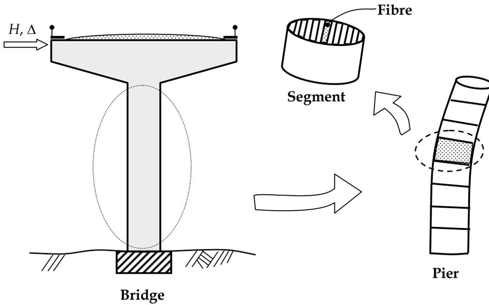
Figure 4: Discretisation of a bridge pier into segments, and further, segments into fibres.
