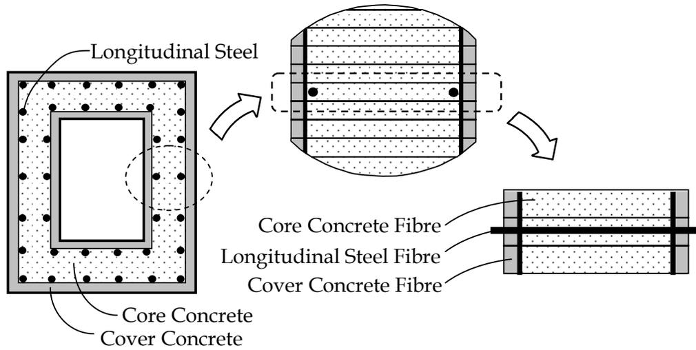
**Figure 5:** Discretisation of a hollow rectangular RC section into concrete (core and cover) and longitudinal steel fibres.
