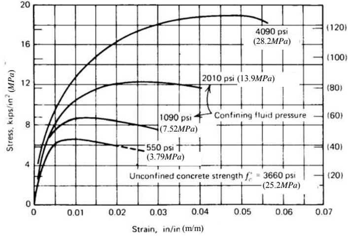
Figure 3: Experimental stress-strain curves of concrete under various confining pressures [Scott *et al.*, 1982].
