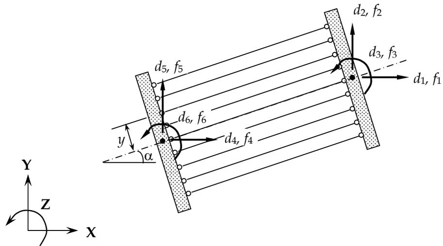
**Figure 6:** End-forces and displacement quantities on a segment in global coordinates.
