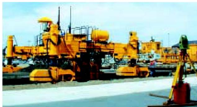
**Figure 12:** Automatically guided slip-form paving machine and on-ground monitoring systems for transferring information from ground to machine. (Source: [www.leica-geosystems.com](http://www.leica-geosystems.com), 2004).
