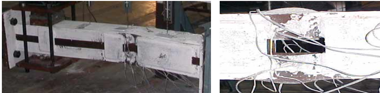
a) Failure of Specimen DC1MB
