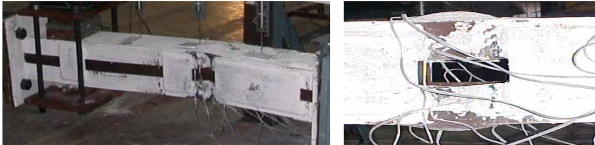
a) Failure of Specimen DC1MB
