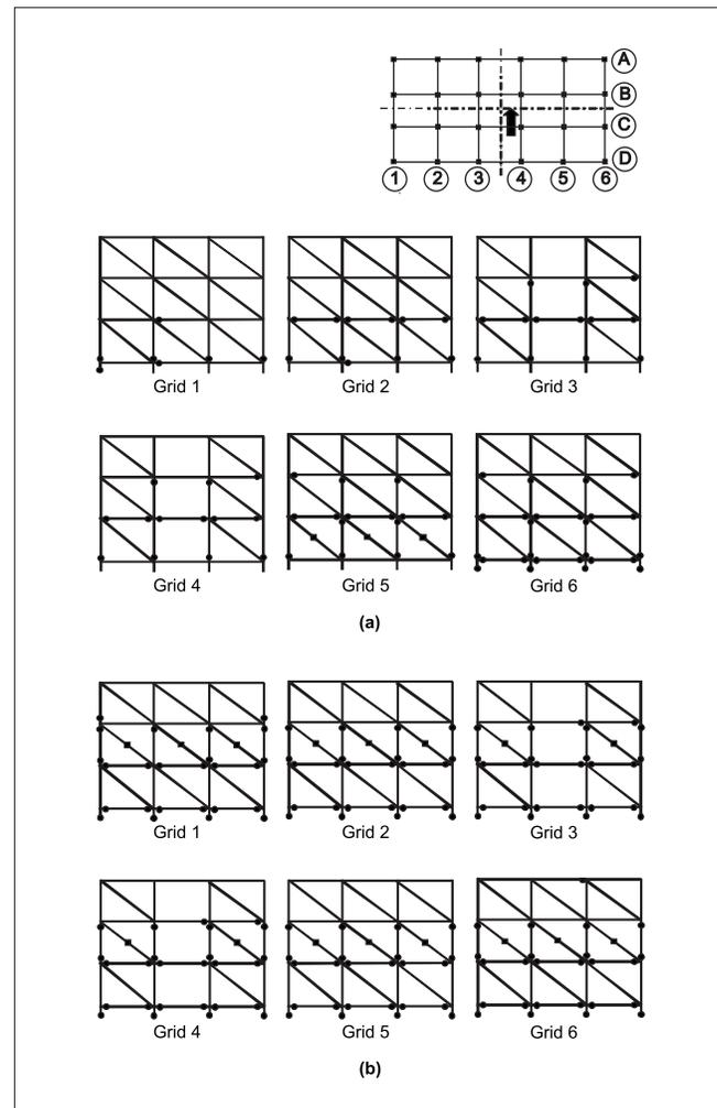
**Fig 7 Location of hinges at failure in the infilled building designed as per (a) IS: 456 and (b) NBC201**
