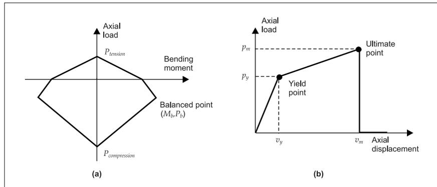
Fig 4 (a) Idealised P-M interaction diagram for the column members; and (b) Axial load displacement curve for equivalent diagonal strut
