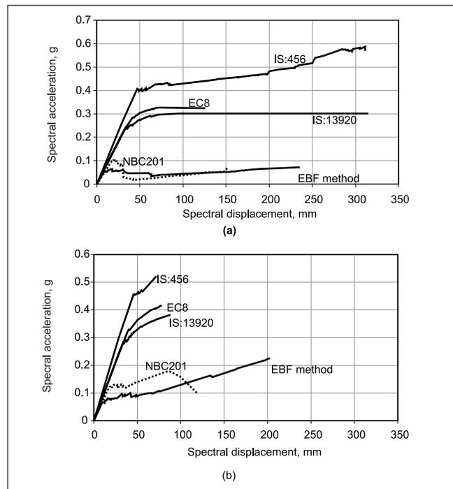
**Fig 6 Capacity spectra of buildings designed by different procedures: (a) Bare frame, and (b) Infilled frame**
