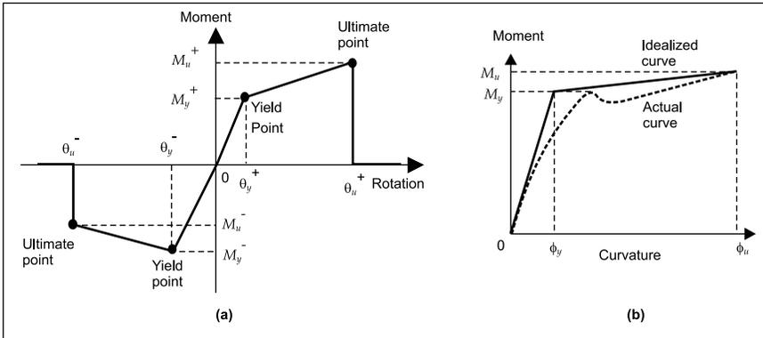
Fig 2 (a) Salient parameters defining the moment-rotation relationship of RC frame members for use in the pushover analysis; and (b) Idealisation of moment-curvature relationship for RC frame members
