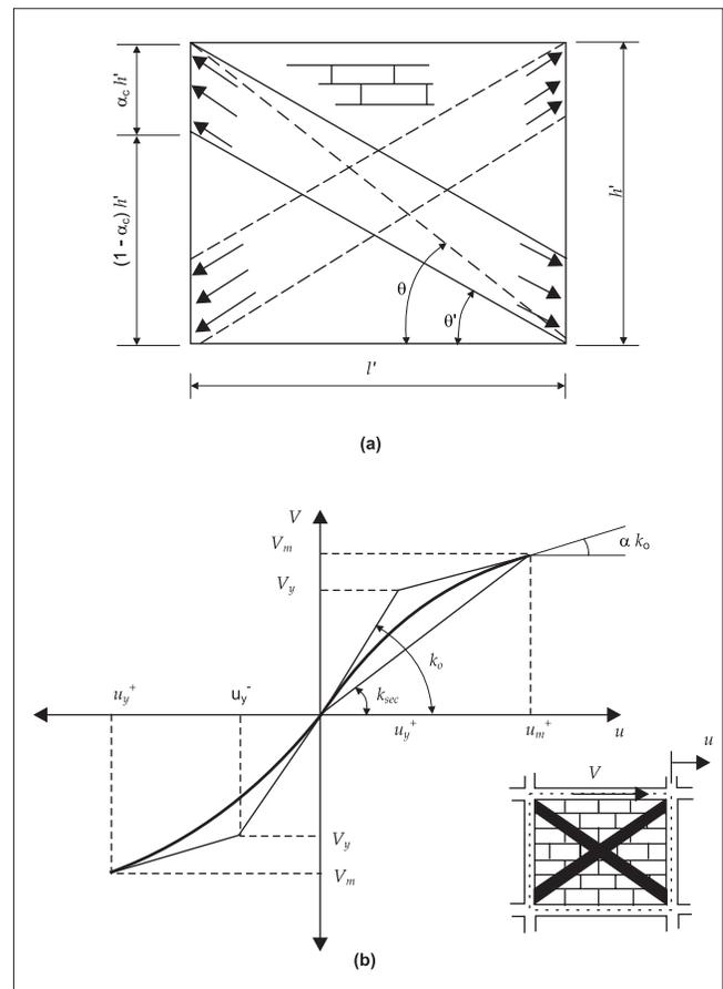
**Fig 1** Equivalent strut idealisation of a masonry infill panel used in the macro-model of infills: (a) Definition of diagonal strut in infill, and (b) Strength envelope for masonry infill panel.
