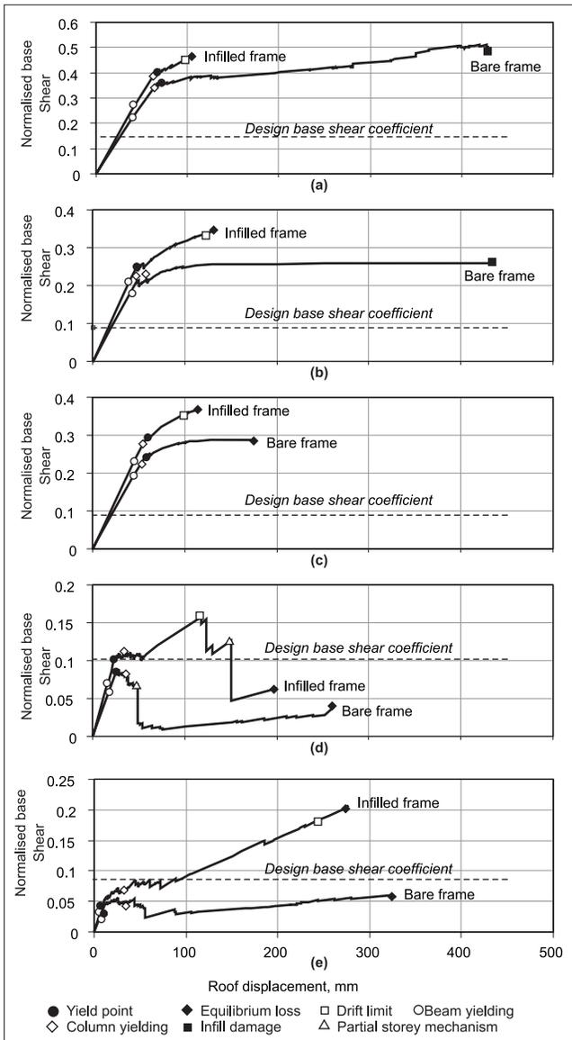
**Fig 5 Capacity curves of buildings designed by (a) IS:456, (b) IS:13920, (c) EC8, (d) NBC201 and (e) EBF method**
