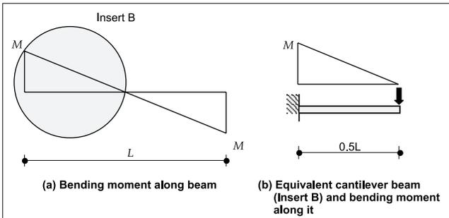
Fig 3 Equivalent cantilever beam idealisation to obtain moment-rotations from moment curvature relations
