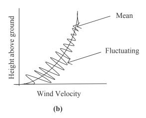
Figure 3: Variation of Wind Velocity with (a) Time, (b) Height
