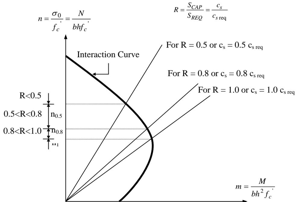
Figure 2: Relation Between Axial Compression Stress, Required Base Shear Coefficient and the Resulting R for a Reinforced Concrete Column
