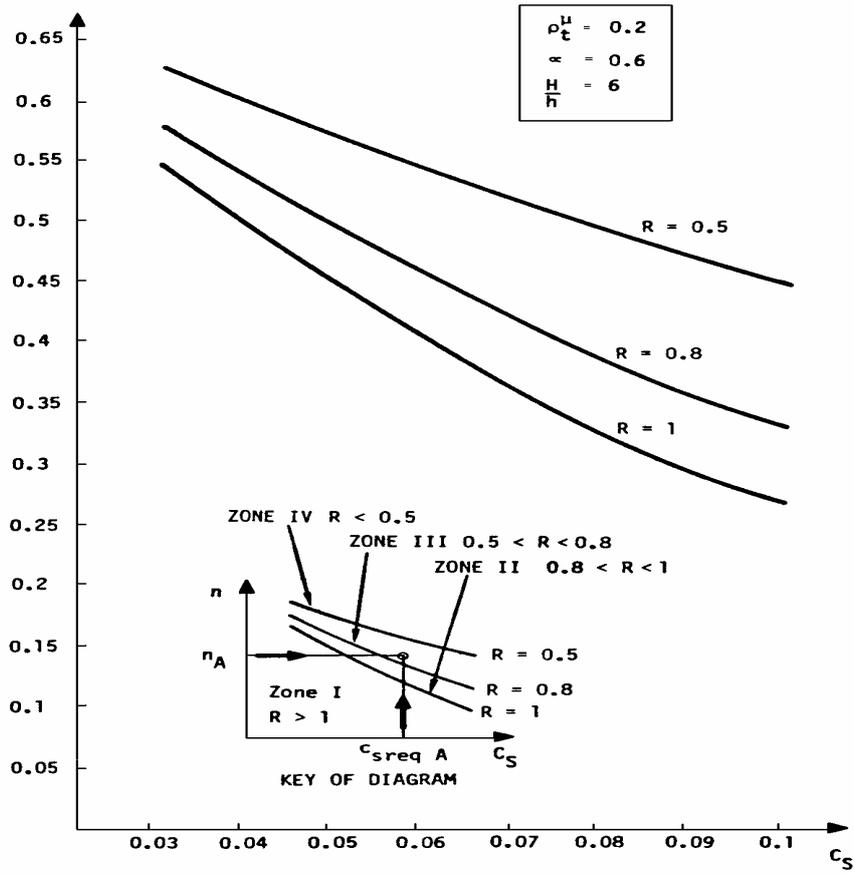
Figure 3: Determination of Strength Index R
