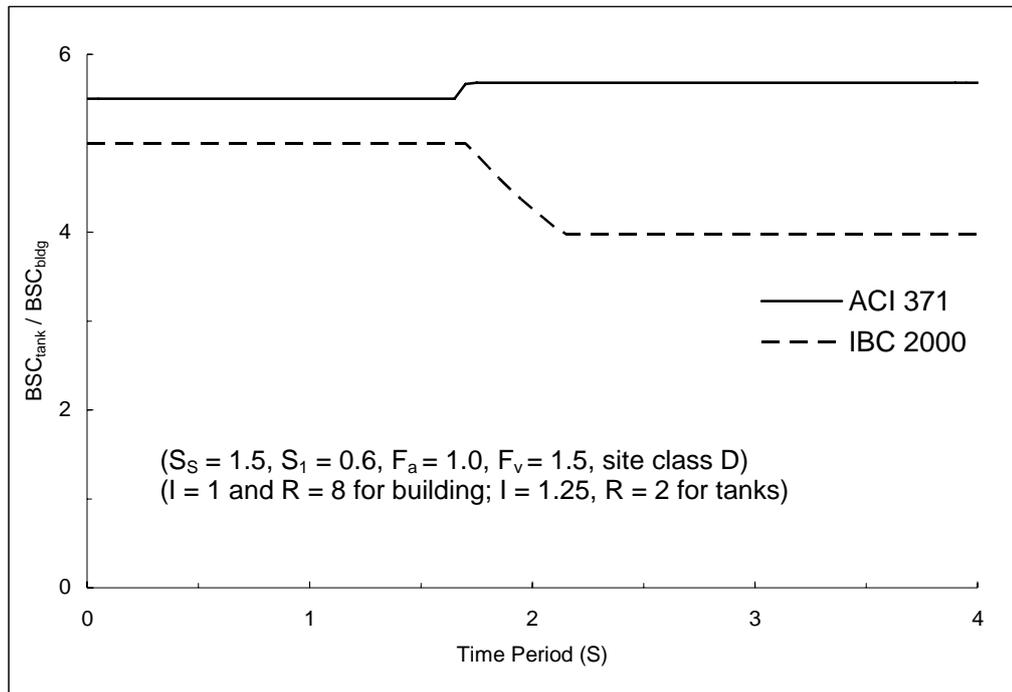
**Figure 5:** Ratio of tank and building base shear coefficient (ACI 371)
