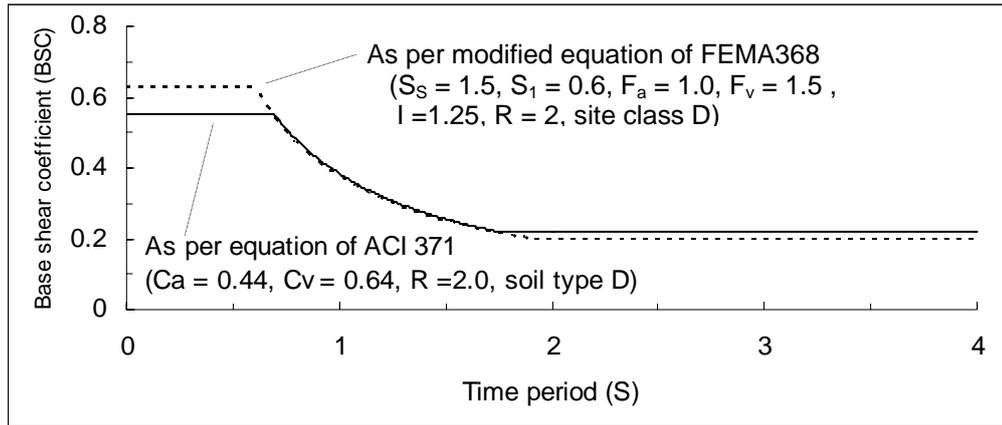
**Figure 3:** Comparison of base shear coefficient from ACI 371 and FEMA 368
