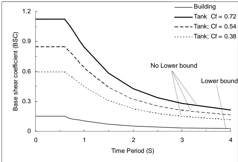
**Figure 17:** Variation of base shear coefficient with time period (NZSEE Guidelines) ( $S_p = 0.67$ ,  $R = 1.0$  for building,  $S_p = 1.0$ ,  $R = 1.3$  for tank,  $Z = 1.2$ ,  $L_u = 1.0$ )
