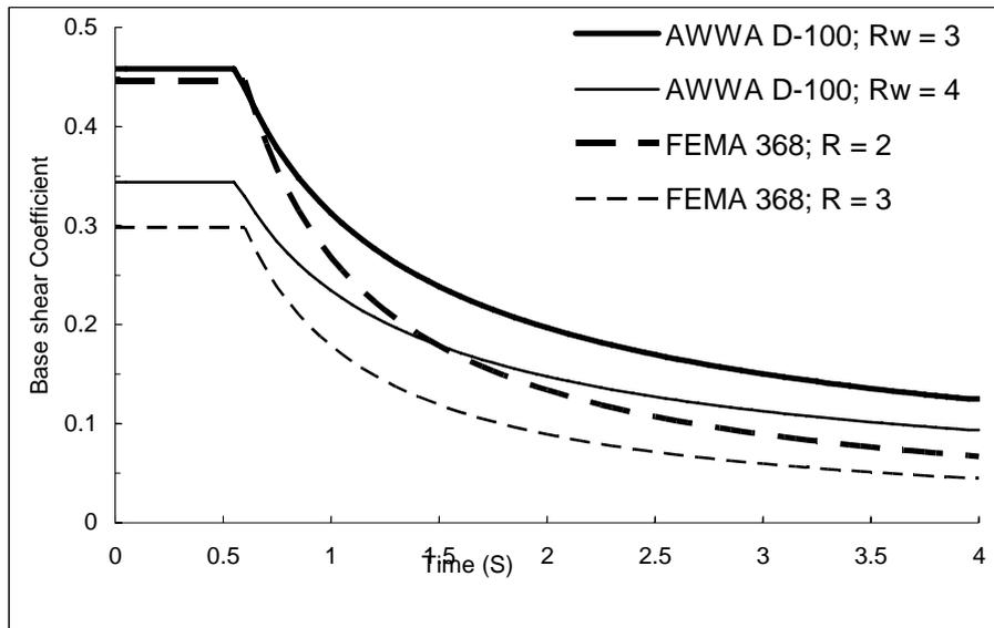
**Figure 9:** Comparison of impulsive base shear coefficient for elevated tank from AWWA D-100 and FEMA 368 (For AWWA D-100  $Z = 0.4$ ,  $S = 1.5$ ,  $I = 1.25$ , soil type C; For FEMA 368:  $S_S = 1.5$ ,  $S_1 = 0.6$ ,  $F_a = 1.0$ ,  $F_v = 1.5$ ,  $I = 1.25$ , site class D)
