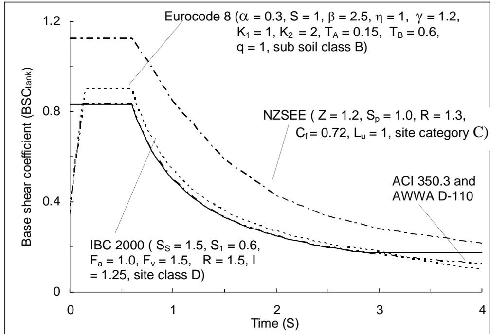
**Figure 20:** Comparison of base shear coefficient for ground supported unanchored concrete water tank obtained from various codes. Most severe zone in each code is considered.
