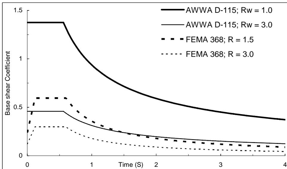
**Figure 13:** Comparison of impulsive base shear coefficient from AWWA D-115 and FEMA368
