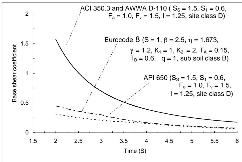
**Figure 23:** Comparison of base shear coefficient for convective mode
