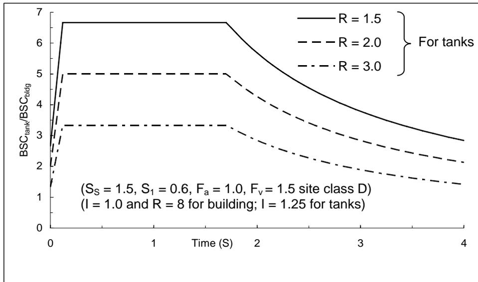
**Figure 12:** Ratio of tank and building base shear coefficient (AWWA D-110)
