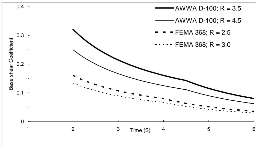
**Figure 8:** Comparison of convective base shear coefficient for ground-supported tank from AWWA D-100 and FEMA 368 (For AWWA D-100  $Z = 0.4$ ,  $S = 1.5$ ,  $I = 1.25$ , soil type C; For FEMA 368:  $S_s = 1.5$ ,  $S_1 = 0.6$ ,  $F_a = 1.0$ ,  $F_v = 1.5$ ,  $I = 1.25$ , site class D)
