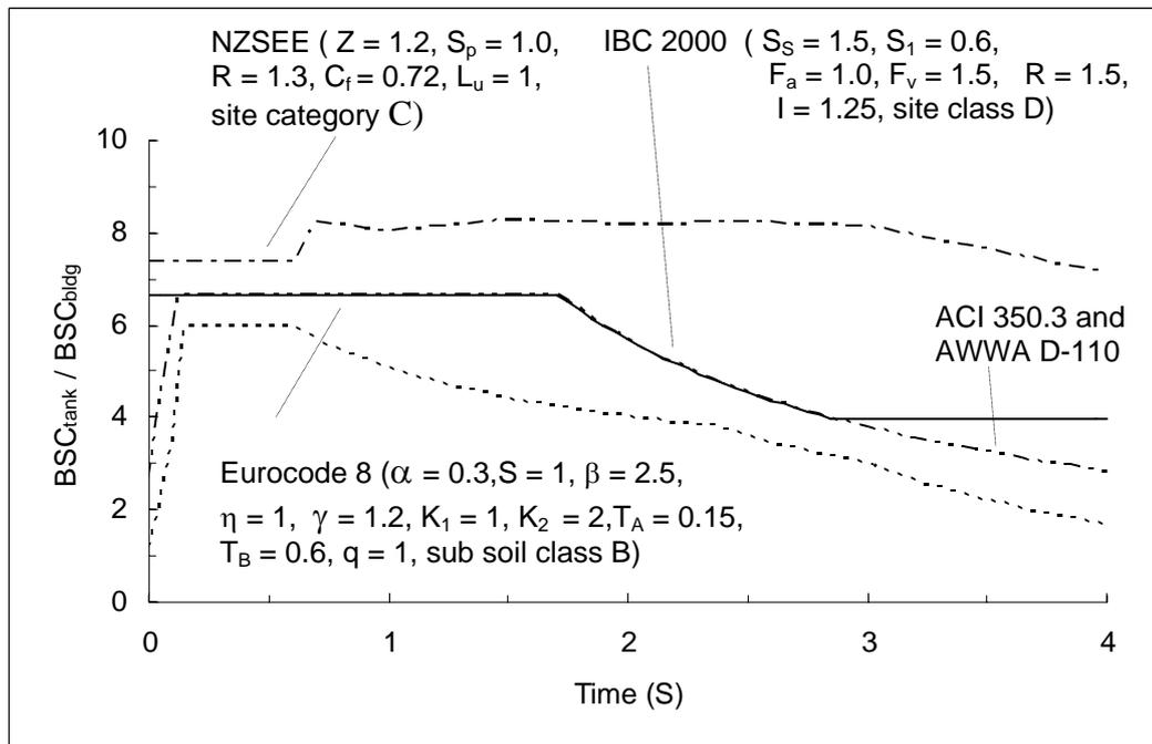
**Figure 21:** Comparison of ratio of base shear coefficients of tank and building from various codes (Low ductility tank).
