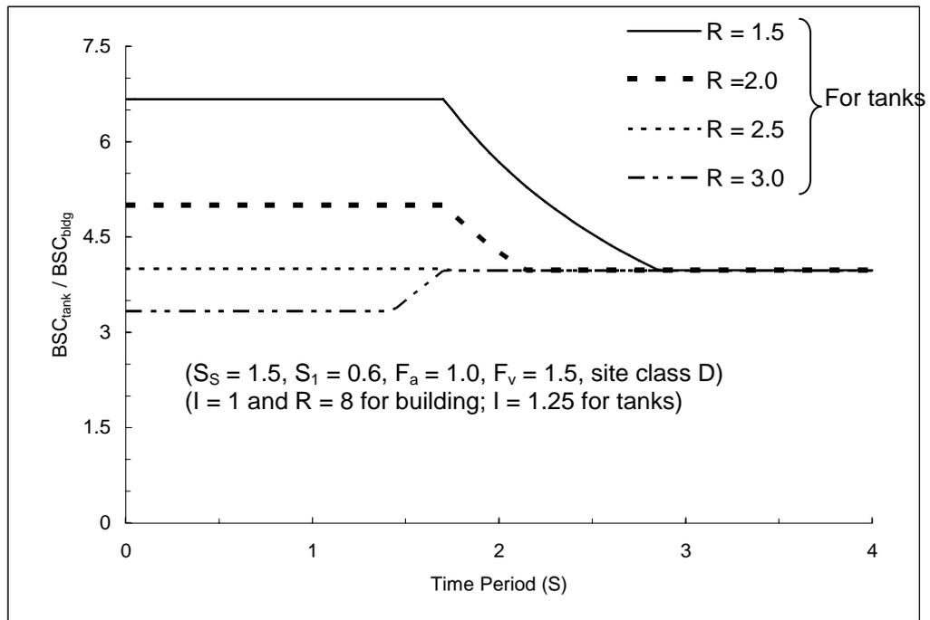
**Figure 2:** Ratio of tank and building base shear coefficient (IBC 2000)
