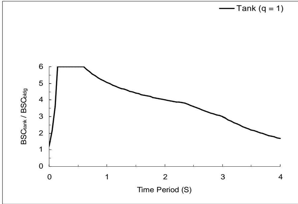
**Figure 16:** Ratio of base shear coefficient of tank impulsive mode and building (Eurocode 8)
