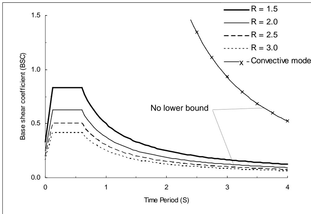
**Figure 6:** Variation of base shear coefficient with time period (ACI 350.3)
