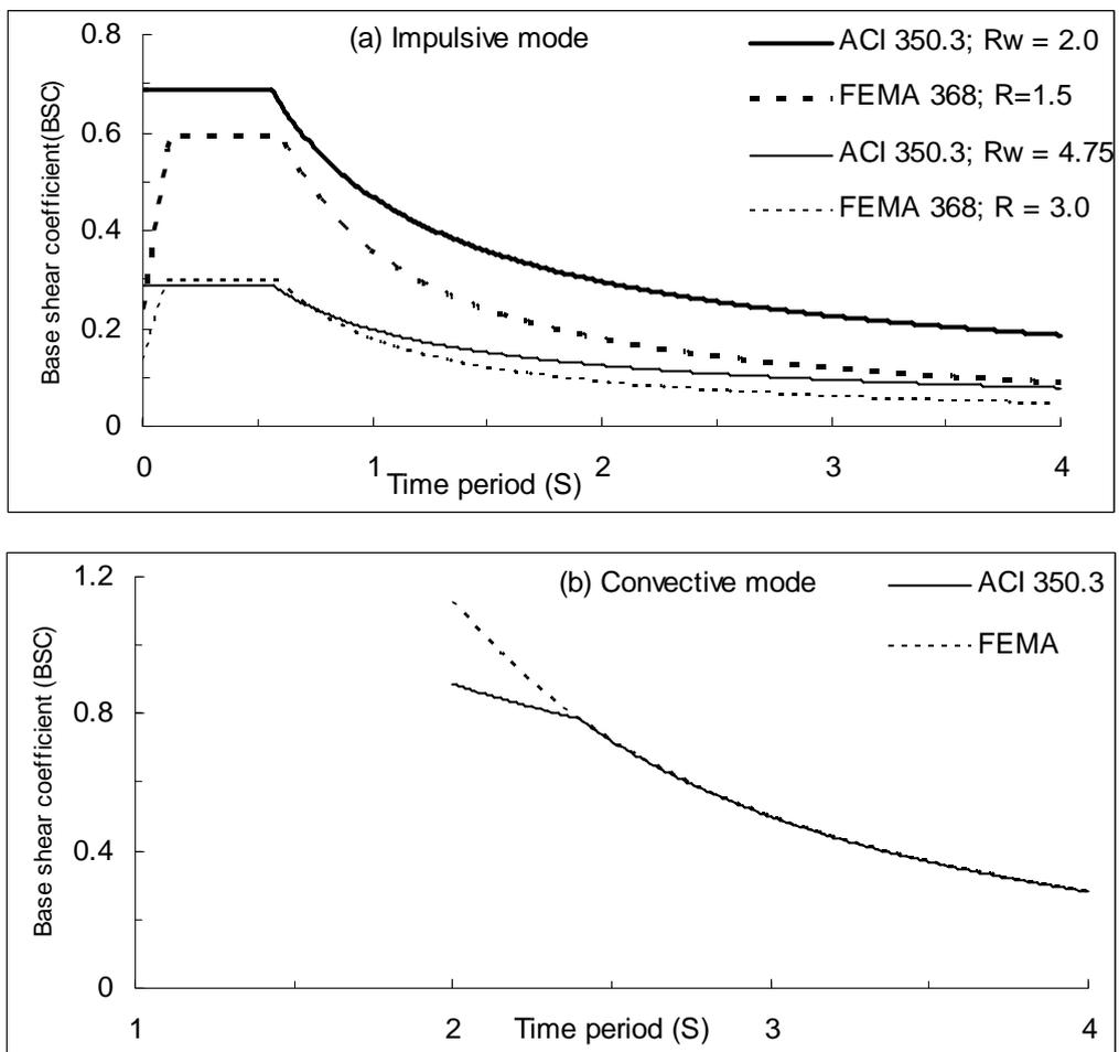
**Figure 4:** Comparison of base shear coefficient from ACI 350.3 and FEMA 368
