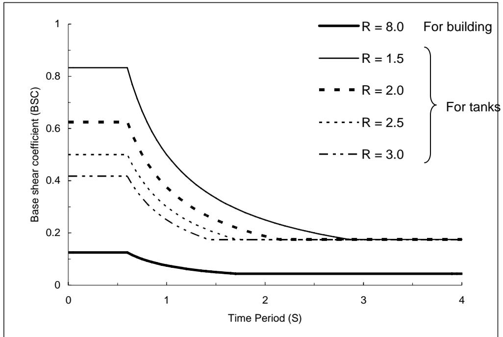
**Figure 1:** Variation of base shear coefficient with natural period;
