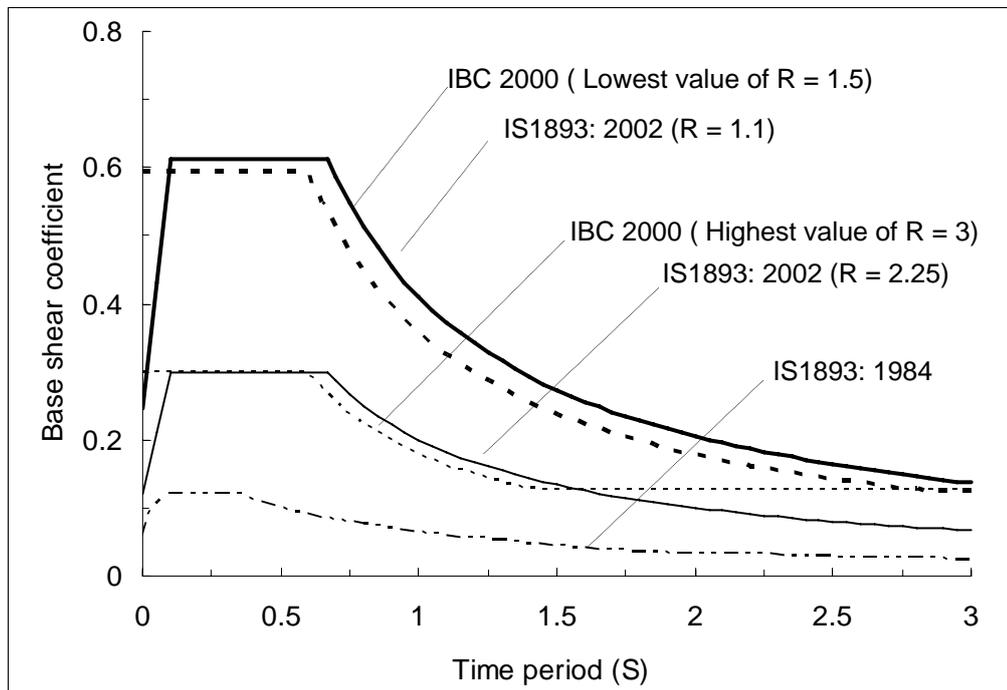
**Figure 25:** Base shear coefficients for tanks from IBC 2000, IS 1893:1984 and IS 1893(Part 1):2002. IBC values are divided by 1.4 to bring them to working stress level.
