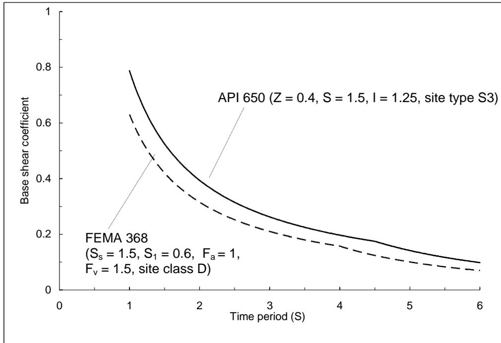
**Figure 14:** Convective base shear coefficient from API 650 and FEMA 368
