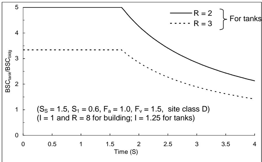
**Figure 10:** Ratio of elevated tank and building base shear coefficient (AWWA D-100)
