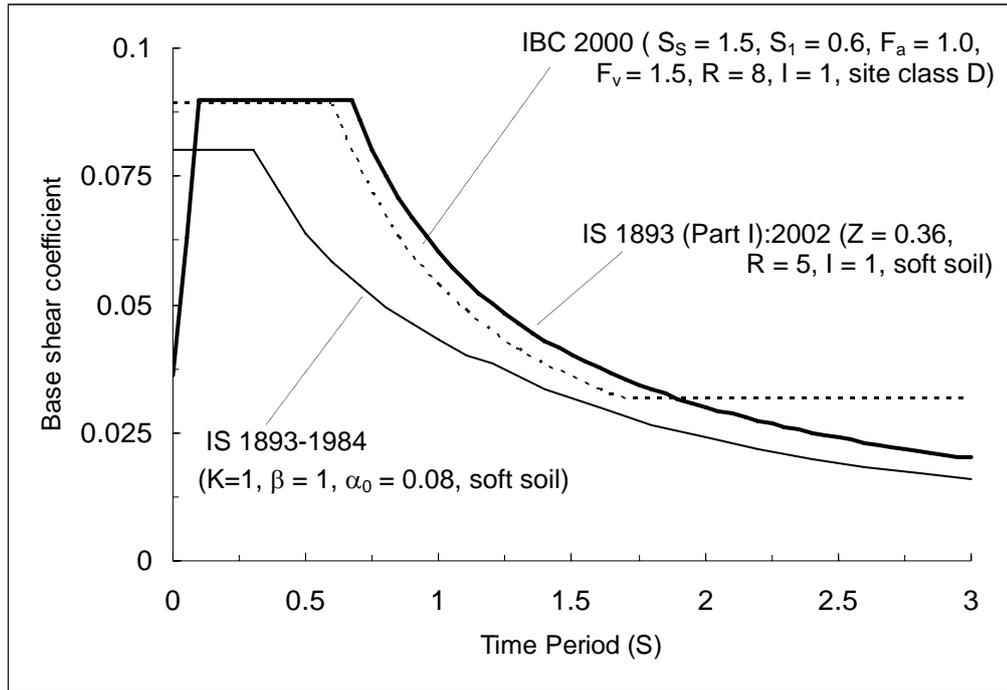
**Figure 24:** Comparison of base shear coefficient for building from IBC 2000, IS 1893:1984, IS 1893(Part 1):2002. IBC values are divided by 1.4 to bring them to working stress level.
