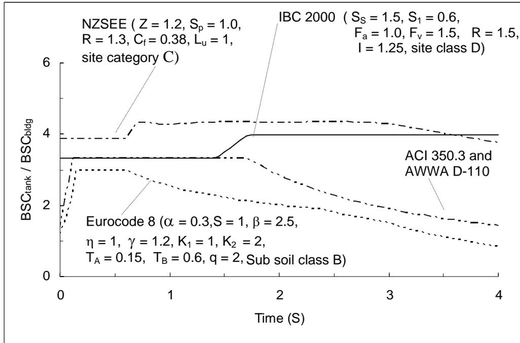
**Figure 22:** Comparison of ratio of base shear coefficient of tank and building from various codes (High ductility tank).
