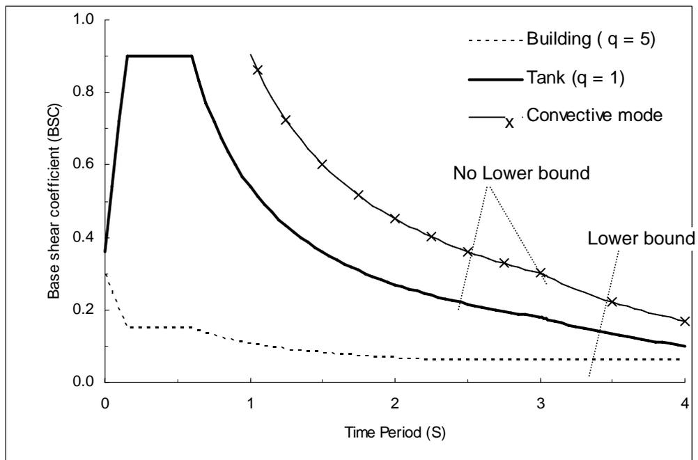
**Figure 15:** Variation of base shear coefficient with time period as per Eurocode 8
