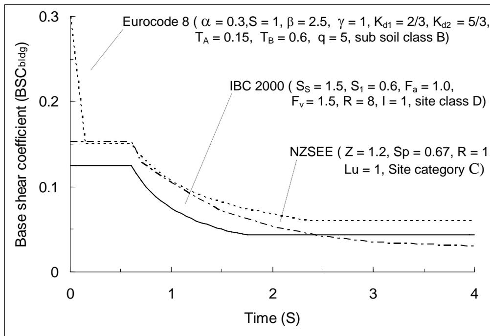
**Figure 19:** Comparison of base shear coefficient for ductile building obtained from various codes. Most severe zone in each code is considered
