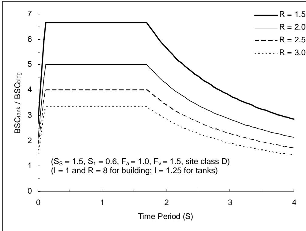
**Figure 7:** Ratio of base shear coefficient of tank (impulsive mode) and building (ACI 350.3)
