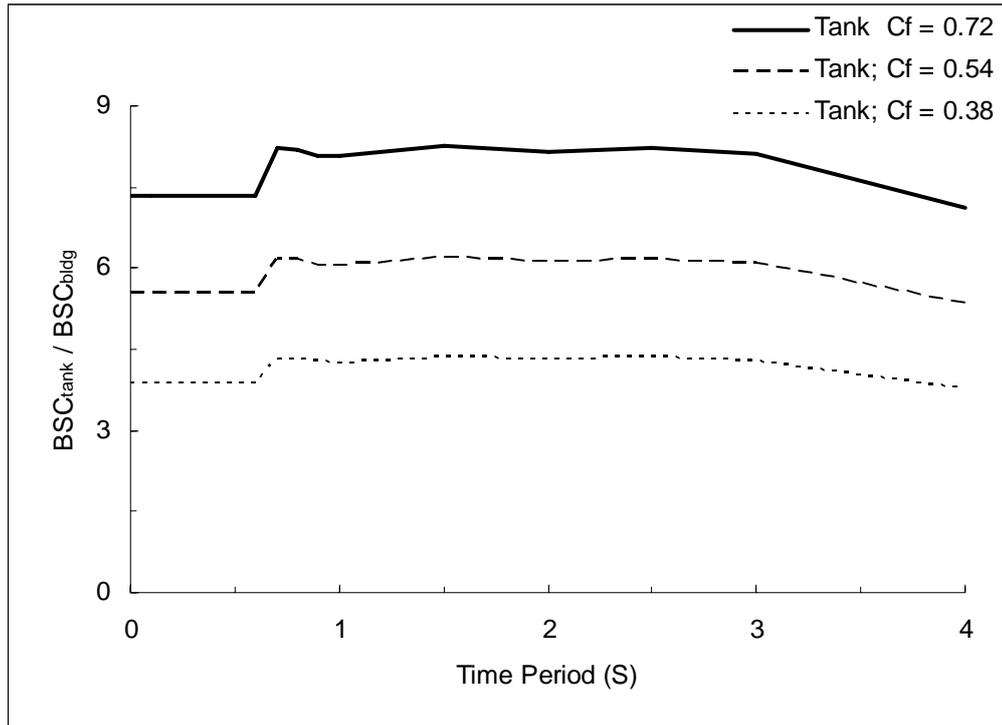
**Figure 18:** Ratio of base shear coefficient of tank and building (NZSEE Guidelines)
