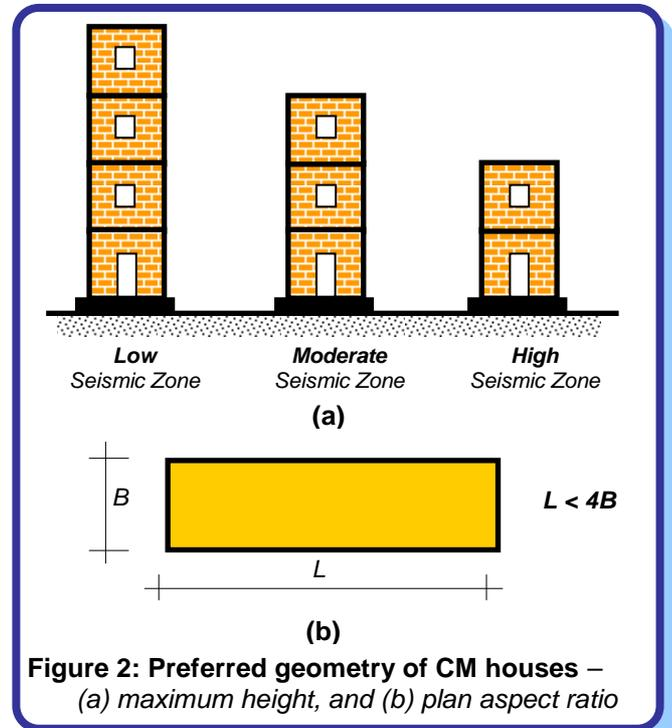
**Figure 2: Preferred geometry of CM houses – (a) maximum height, and (b) plan aspect ratio**
