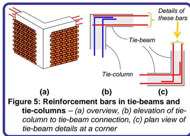
In tie-columns, at least 4 deformed steel bars of 10 mm diameter should be provided, and tied with 6 mm diameter mild steel ties at 200 mm centers (Figure 6a); closely spaced ties are required in top and bottom portion of a tie-column, with spacing of 100 mm. Ties should have 135° hook ends. In RC tie-beams, minimum reinforcement to be provided is somewhat similar.
