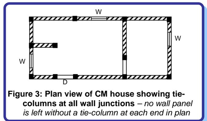
**Figure 3: Plan view of CM house showing tie-columns at all wall junctions – no wall panel is left without a tie-column at each end in plan**
