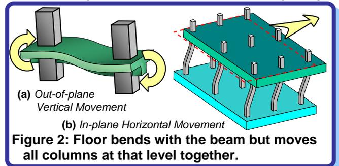
Figure 2: Floor bends with the beam but moves all columns at that level together.
