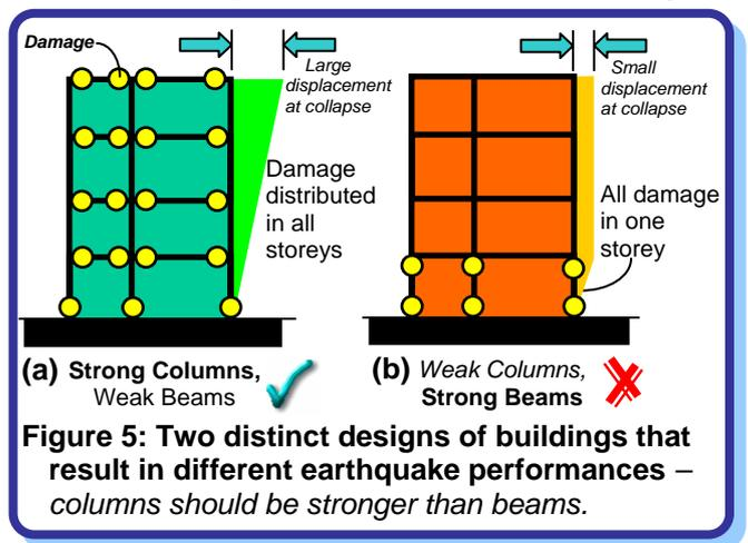
**Figure 5: Two distinct designs of buildings that result in different earthquake performances – columns should be stronger than beams.**
