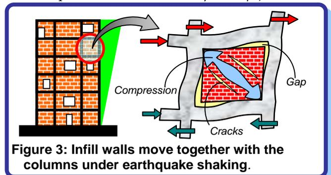
Figure 3: Infill walls move together with the columns under earthquake shaking.
