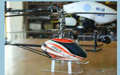
Vibhram is an innovative and improved helicopter design, making use of dissimilar coaxial rotors mounted above the body of the helicopter. This concept has been predicted to be 10-20 per cent more efficient than existing helicopter designs like the conventional (single main rotor and tail rotor) and the regular coaxial helicopters. The team behind this design consisted of MTech and PhD students from IIT Kanpur, who were advised by Dr. Abhishek, Department of Aerospace Engineering, IIT Kanpur.
