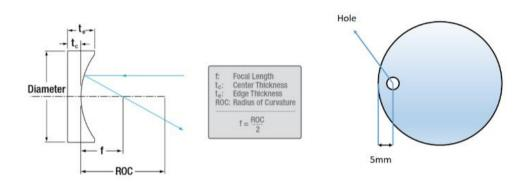
Plano-concave mirror for 532nm of diameter=100mm, f=150mm, ROC= 300mm, tc =12mm, te=16.2mm Qty:2 with hole of diameter 5mm, hole center located 5mm from periphery
