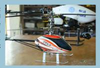
Vibhram is an innovative and improved helicopter design, making use of dissimilar coaxial rotors mounted above the body of the helicopter. This concept has been predicted to be 10-20 per cent more efficient than existing helicopter designs like the conventional (single main rotor and tail rotor) and the regular coaxial helicopters. The team behind this design consisted of MTech and PhD students from IIT Kanpur, who were advised by Dr. Abhishek, Department of Aerospace Engineering, IIT Kanpur.
