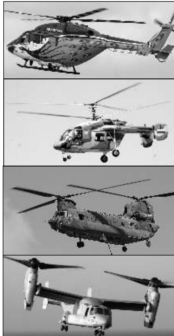
Fig 2: (From top to bottom) Conventional rotor, Coaxial rotor, Tandem rotor and Tilt rotor.
