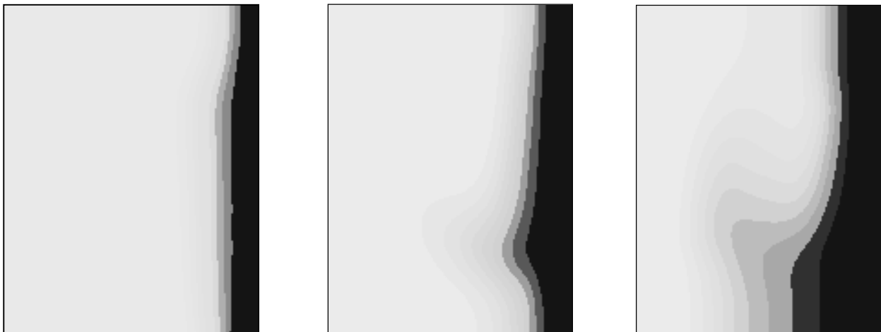
Figure 3 Solid-liquid interface at different timesteps Ra=2.5e5
