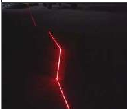
Fig.2: Image of a laser line on an uneven surface
